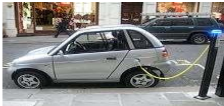
Fig. 5 Electric Reva/G-Wiz I Car Charging a Battery at an Electric Charging Station (Roadside City of London)
