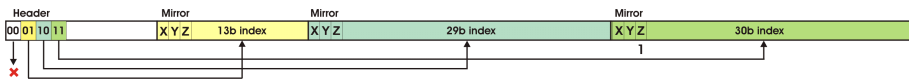
Figure 3. Symmetry-aware Sparse Voxel Directed Acyclic Graph (SSVDAG) binary representation of inner nodes with short, long and extra-long pointers to the child nodes
