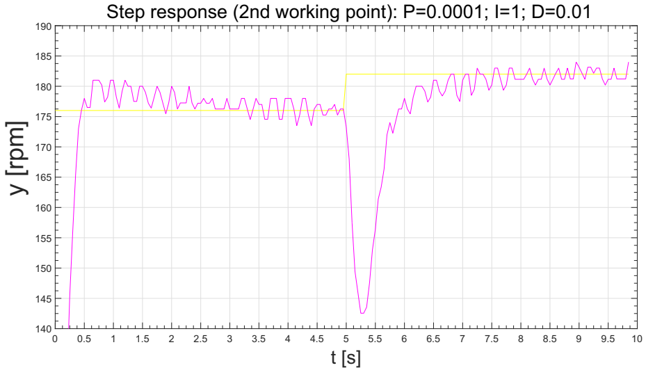
Figure 16. Step response (closed loop) – 2 nd working point – under inappropriate controller
