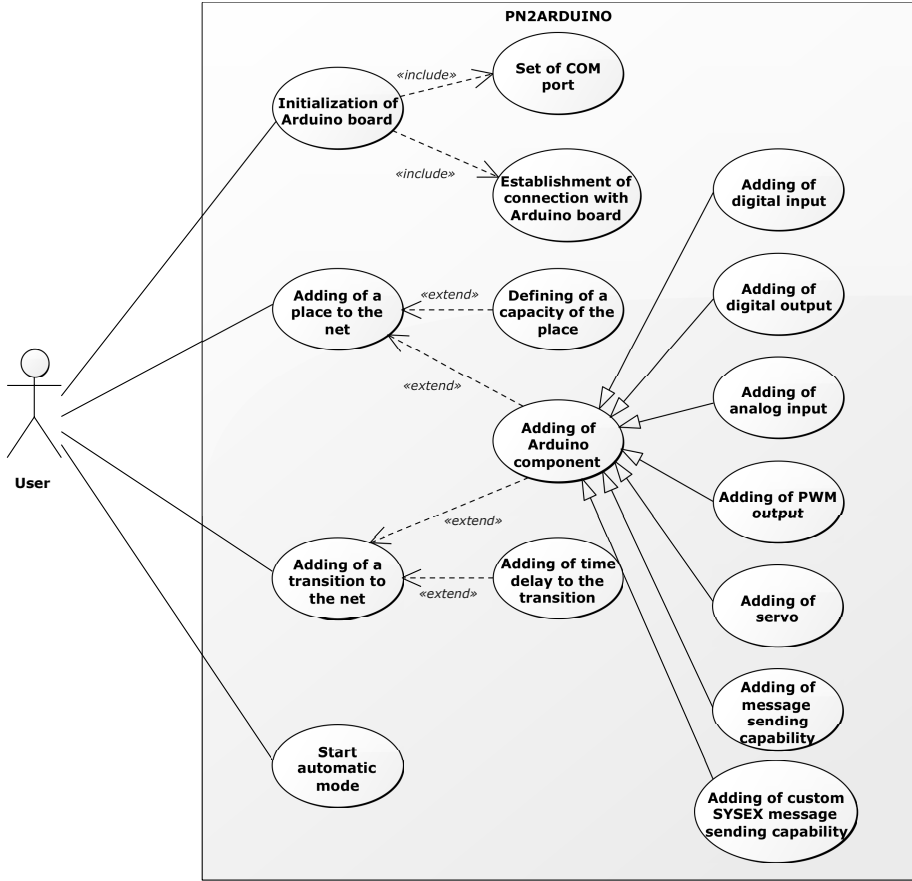
Figure 3. PN2ARDUINO – use-case diagram
