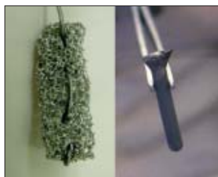
Fig. 2 Al foam cathode (left) and the Pu metal anode (right).
