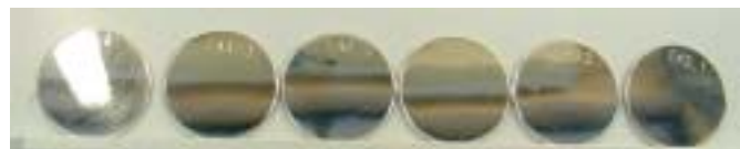
Fig. 7.5 Plutonium containing neutron sources for testing waste assay systems at their lower limit of detection
