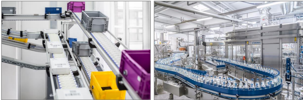
Figure 1: Complex sliding chain conveyor systems; left: Bosch Rexroth [16], right: Kronos AG [17]
