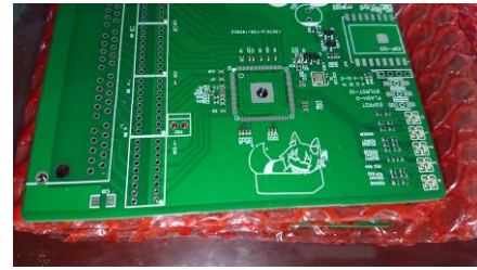
Figure 4 The PCB with some SMT components soldered
