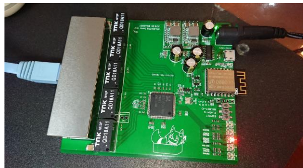
Figure 1 The working ethernet switch
