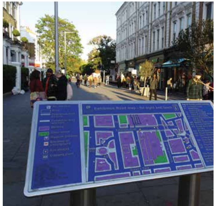
Reflection: Exhibition Road continues to be an innovative and successful public space that relies on the considerate interaction between its various users. The absence of signal-controlled crossings presents risks to partially sighted or blind individuals. Nevertheless, tangible efforts have been made to mitigate these risks through the provision of braille signage and maps.
