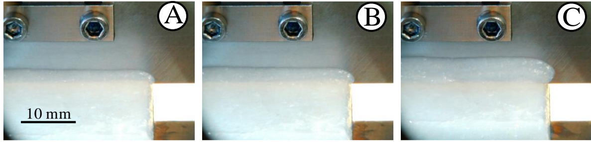
Fig. 3.17. Images of petroleum jelly subject to interrupted scraping, taken at times labelled A, B and C in Fig. 3.16(a,i). Conditions: \delta_0 = 5 mm, s = 1 mm, V = 1 mm/s, scraping time = 5 s, and relaxation time = 60 s.
