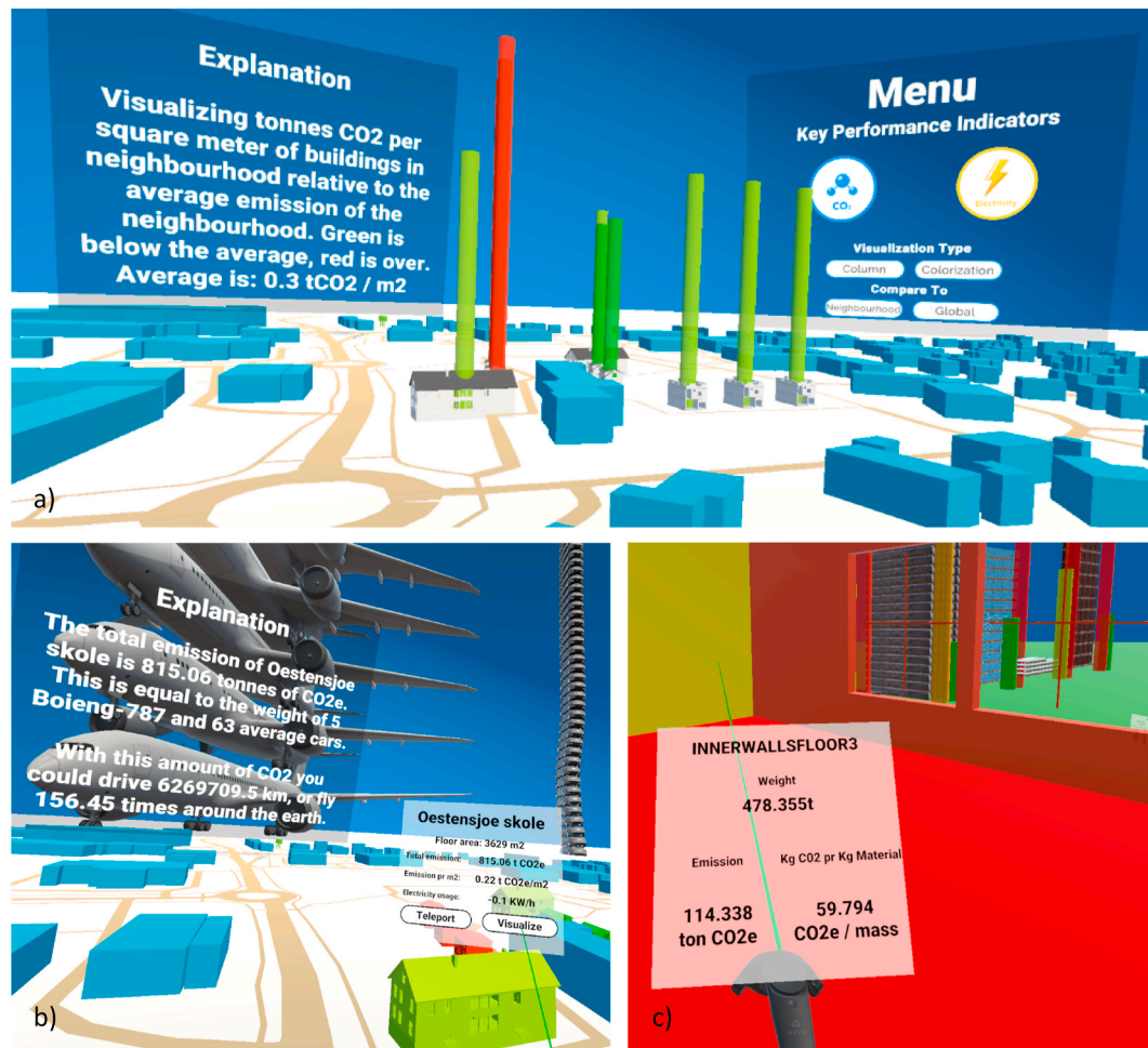
Fig. 7. Snapshots using VR to visualise GHG emissions of buildings [93] using a) red and green columns to show being below or above a threshold, b) airplane icons to relate GHG emissions of a building to flying, c) a colour code to visualise the impact of building elements. (For interpretation of the references to colour in this figure legend, the reader is referred to the Web version of this article.)
