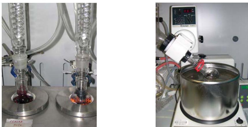
Picture 1: Various steps of method EN 14362: a) extraction; b) concentration.
