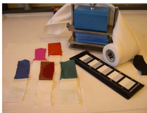
Picture 5: Perspirometer, multifibre adjacent fabric, grey scale for method EN ISO 105-E04.
