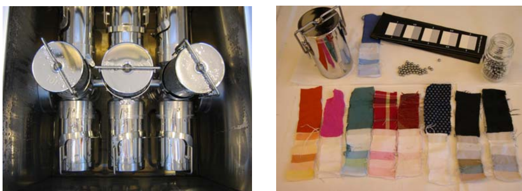
Picture 4: a) Gyrowash apparatus; b) sample vessel for Gyrowash, grey scale, steel balls and washed specimens.
