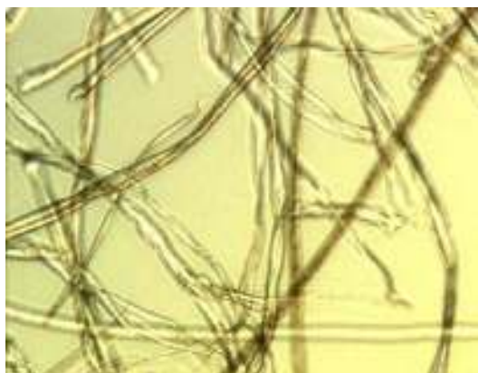
Fig. 1: 40.2% poly(lactide) – 59.8% cotton (sample 025 ). 250X.
