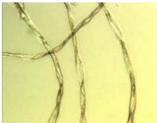
Fig. 2: Residue of cotton after dissolution of poly(lactide) (sample 016 ). 250X.
