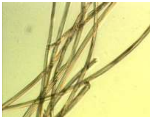
Fig. 5: Residue of viscose after dissolution of poly(lactide) (sample 033 ). 250X.
