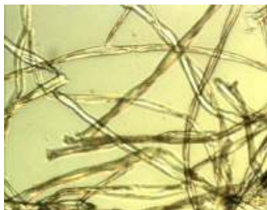
Fig. 3: Residue of cotton after dissolution of poly(lactide) (sample 017 ). 250X.
