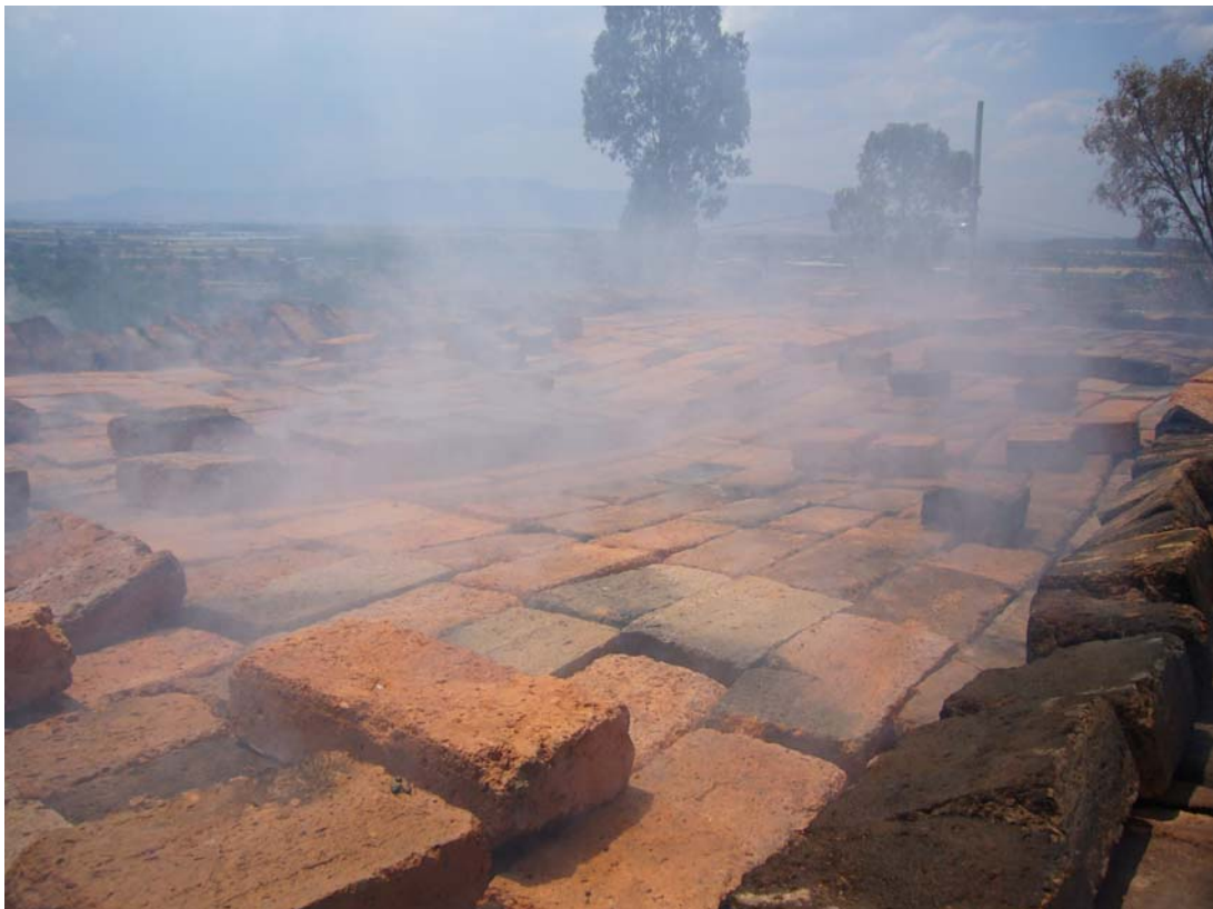
Photo 5: View on the top of a stationary kiln in the initial burning phase
