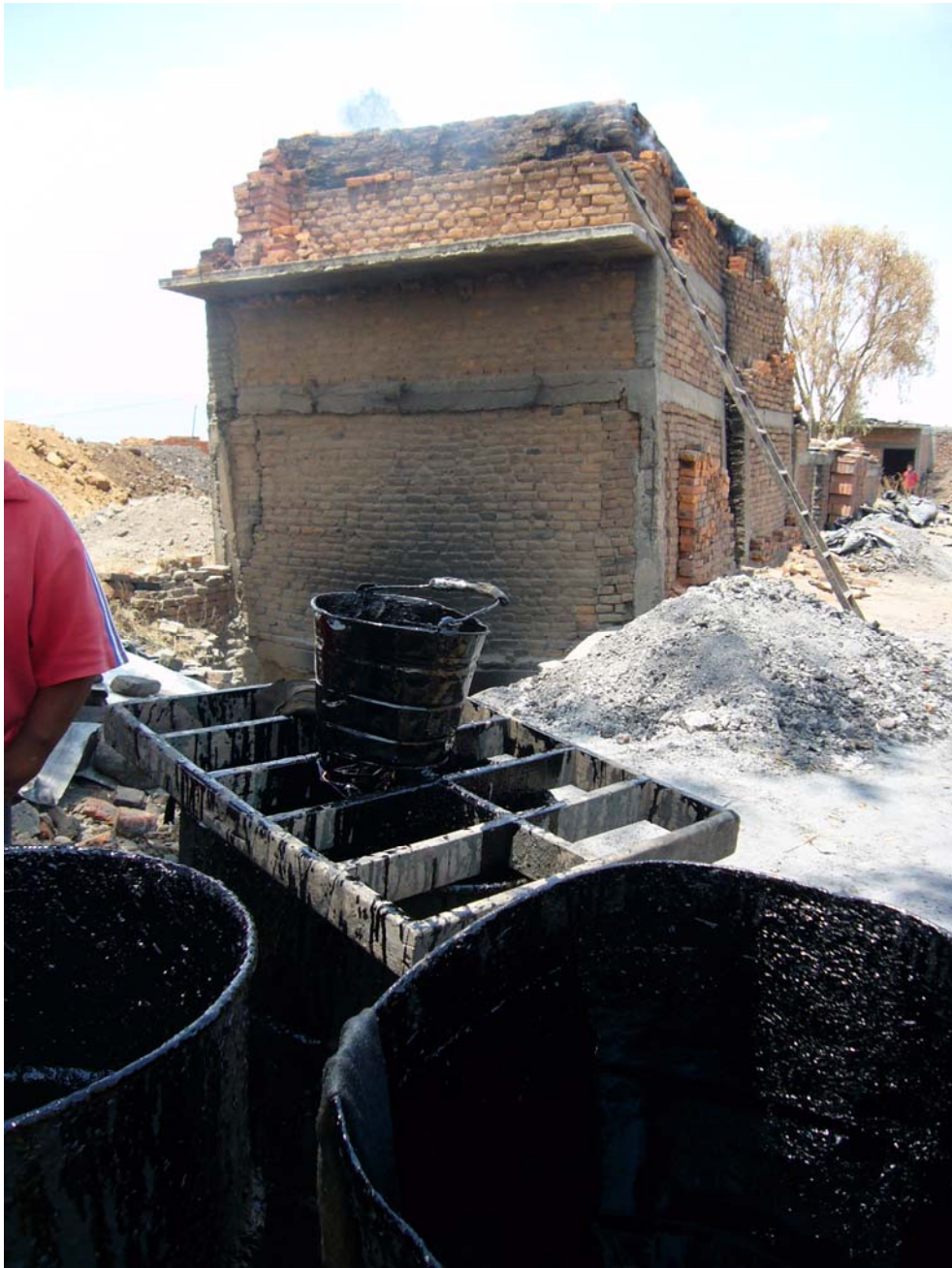
Photo 10: Brick 2, Stationary kiln, fuel (tar) and ashes visible
