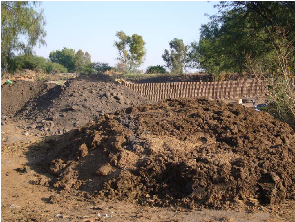
Photo 14: Brick 5. Clay and dung used for brick production
