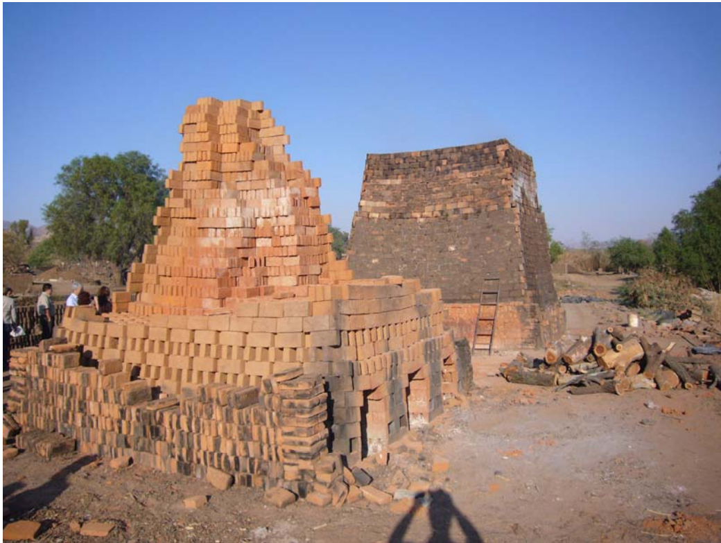
Photo 17: Brick 5. First kiln under demontage (red bricks), second kiln sealed with dung and ready to burn
