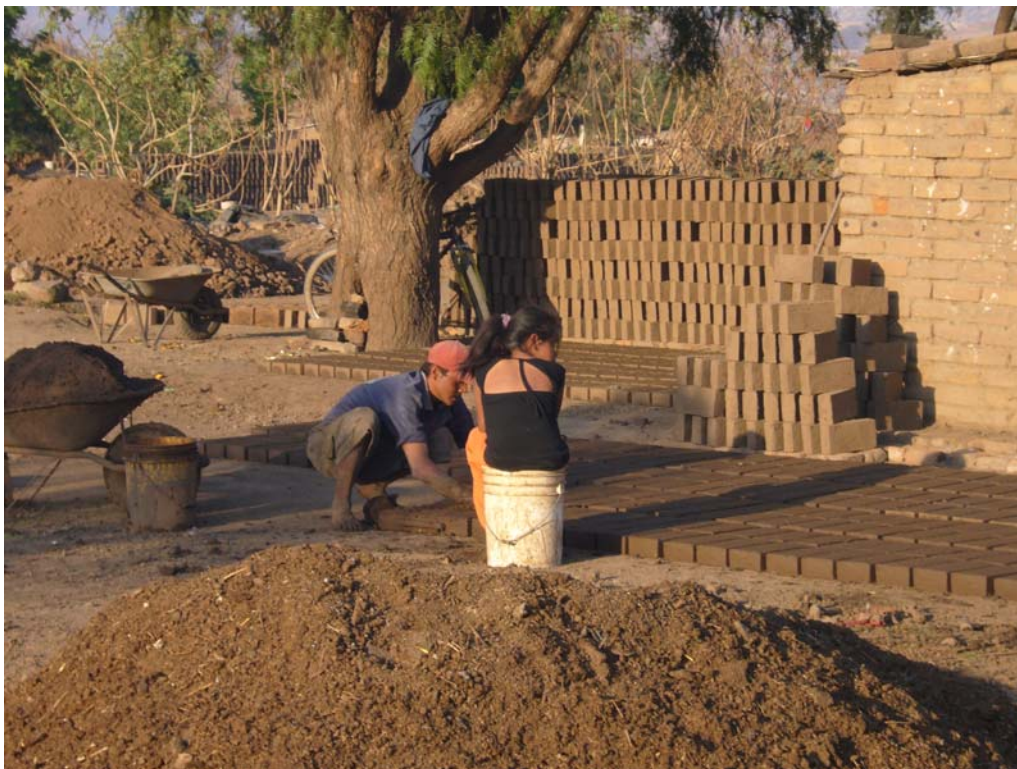
Photo 13: Brick 5. Drying of the raw bricks and ingredients
