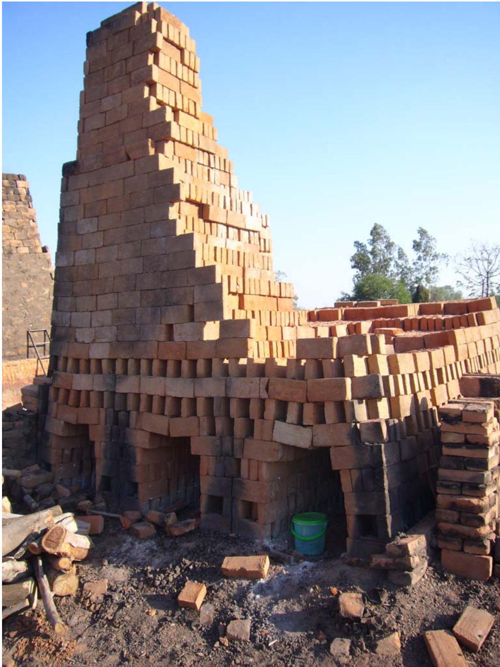
Photo 15: Brick 5. Mobile brick kiln with burnt bricks under de assembling
