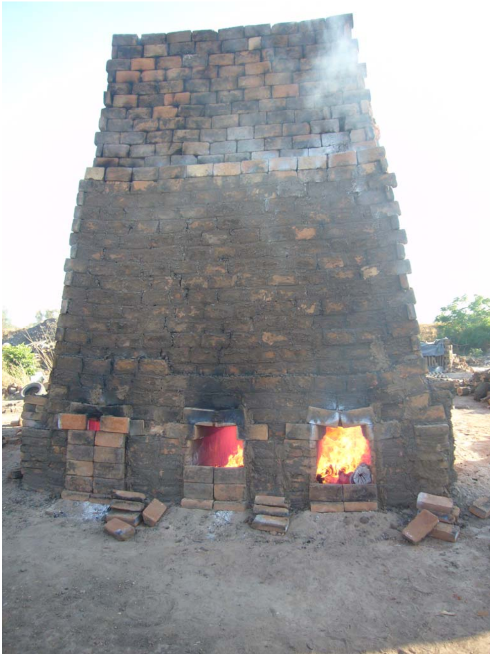
Photo 16: Brick 5. Mobile kiln under fire
