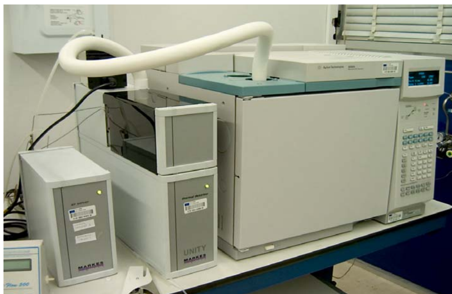
Figure 55 – Chromatography analysis (2D-GC)
