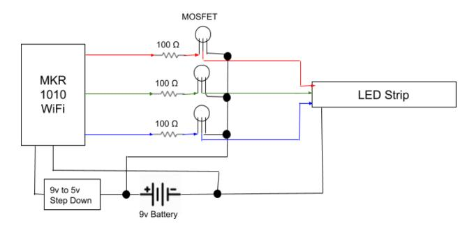
Figure 3 - Diagram of the Arduino to LED Circuit
