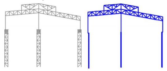
**Figure 16.** Models for calculating columns. Model No. 1 (left) is presented in the article; model number 2 - classic
