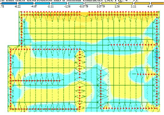
Figure 4. Isofields of stresses according to  $M_y$  in the case of calculating the floor slab when constructing the design model of the building frame (case 1).
