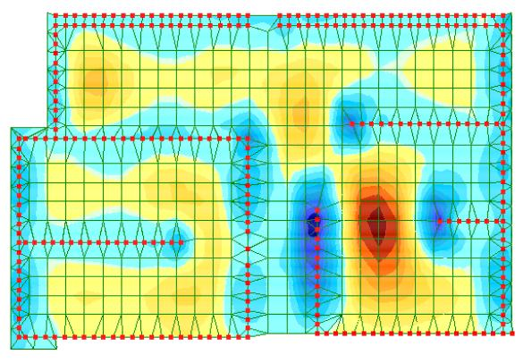
**Figure 7.** Isofields of stresses in  $M_x$  in the case of cutting a floor slab from the building frame (case
