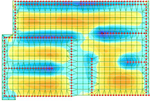
**Figure 6.** Isofields of stresses according to  $M_y$  in the case of cutting the floor slab from the building frame (case 2)
