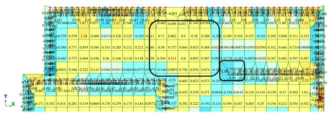
**Figure 13**. Part of the stress mosaic by  $M_x$  in the case of calculating the floor slab as part of the building frame (case 1)
