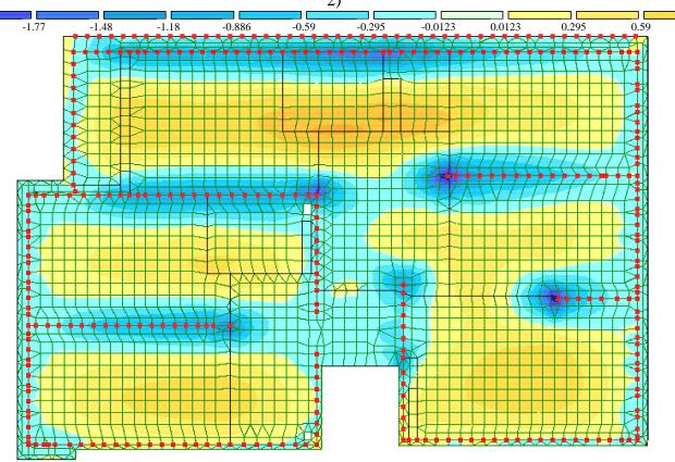
Figure 8. Isofields of stresses according to  $M_y$  in the case of a separate calculation of the floor slab (case 3)
