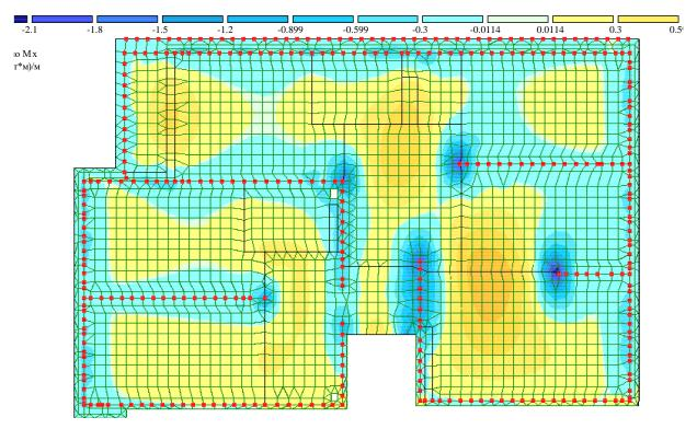
**Figure 9.** Isofields of stresses by  $M_x$  in the case of a separate calculation of the floor slab (case 3)
