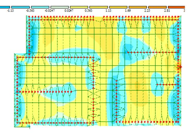
**Figure 5.** Isofields of stresses in  $M_x$  in the case of calculating a floor slab as part of a building frame (case 1)
