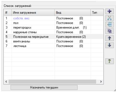
**Figure 3**. List of load cases in the case of drawing up a design model for an individual slab (case 3)
