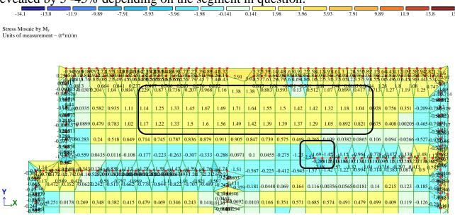
**Figure 10.** Part of the stress mosaic according to  $M_y$  in the case of calculating the floor slab as part of the building frame (case 1)
