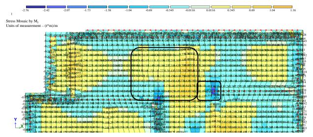
**Figure 15**. Part of the stress mosaic by  $M_x$  in the case of a separate calculation of the floor slab (case 3)
