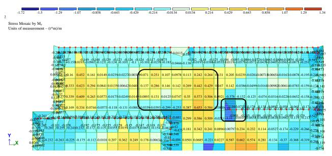
**Figure 14.** Part of the stress mosaic by  $M_x$  in the case of cutting a floor slab from the building frame (case 2)
