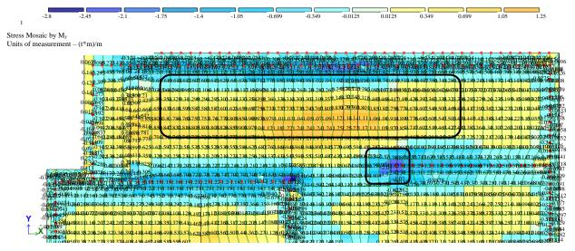
**Figure 12.** Part of the stress mosaic by  $M_y$  in the case of a separate calculation of the floor slab (case 3)
