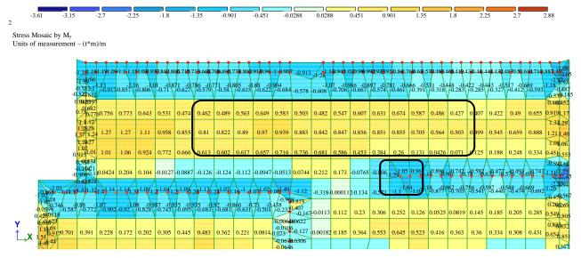
**Figure 11.** Part of the stress mosaic according to  $M_y$  in the case of cutting out a floor slab from the building frame (case 2)
