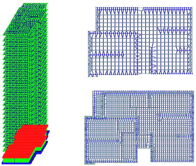
**Figure 1.** The design model of the building frame, the design model of the slab cut from the building frame, and the design model of the slab compiled separately (the location of the calculated floor slab is highlighted in red).
