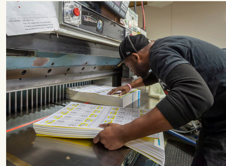
An employee feeds stacks of coated paper into a notebook cutting machine. Credit: South Sound Business Journal
