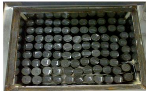
Fig.3.3: Samples Are Cured At Different Temperature with Wax Coating
