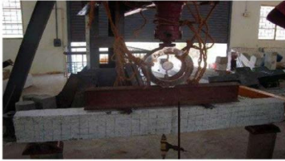
Fig. 4.1 General View of Failure Pattern of Control RC Beam
