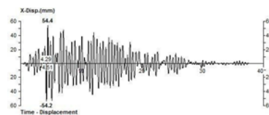
Fig 4.1: Time History of Storey (1 st Floor) Displacement (a) Present FEM (b) STAAD Pro for 15° slope.
