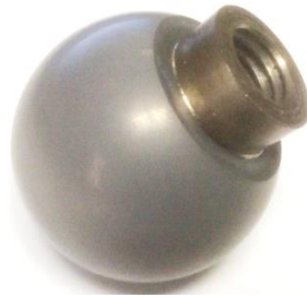
Fig. 8 Alumina ceramic head with titanium sleeve brazed
