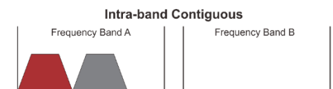
Gambar 1. Skenario Carrier Aggregation Intraband, Contiguous
