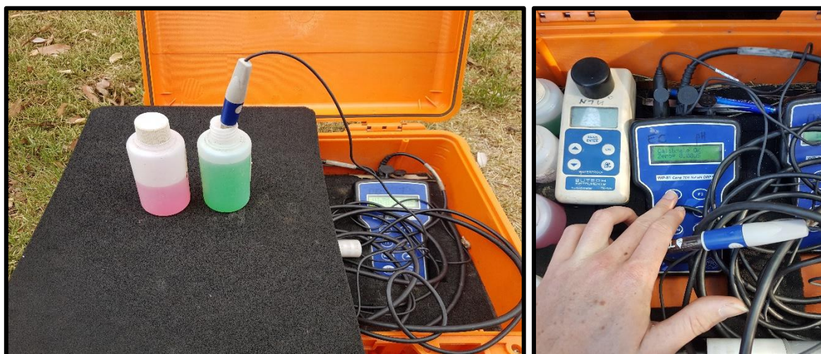
Figure 6: Photos showing part of the calibration process for field meters (Benjamin Green 2019).
