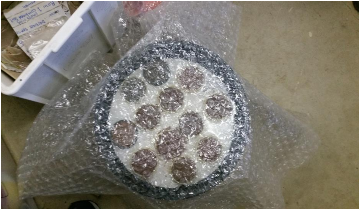
Figure 3. 10: Sample rings covered with plastic to inhibit evaporation after soaking
