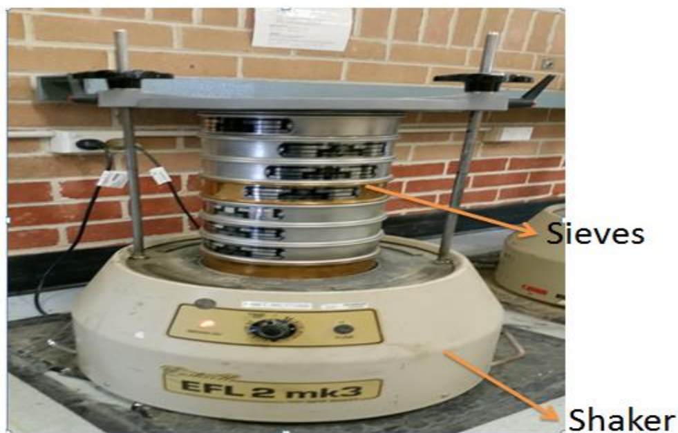
Figure 3. 8: Mechanical analysis of a soil sample
