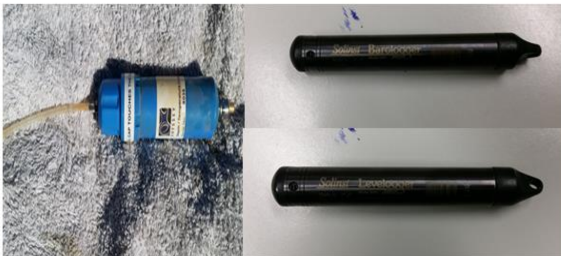
Figure 3. 14: Different loggers deployed in the boreholes
