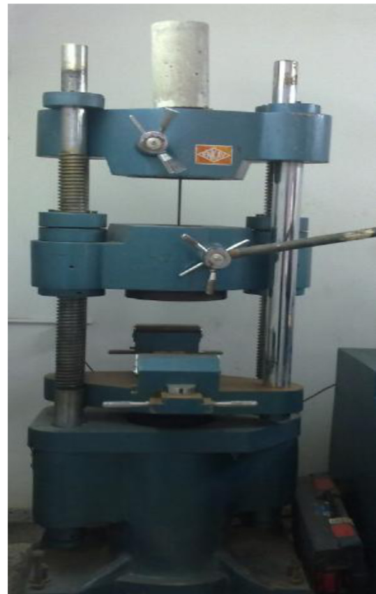
Fig. 3. Pull-out testing machine.
