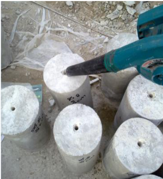
Fig. 2. Cleaning of the drilled holes.
