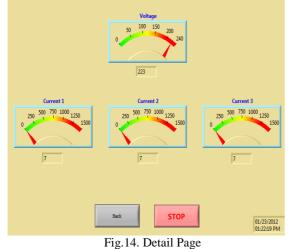
Press Back button to go back to the system monitor. There are three details button beside generators. These buttons will move you the page contain the status of generators and its specifications.
