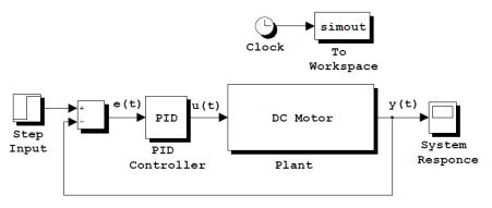
Figure 3.4: SIMULINK model of PID controller
