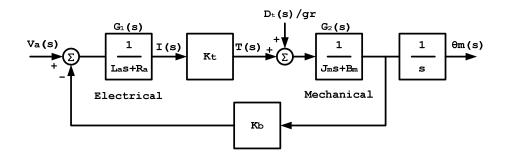
Figure 2.3: Block diagram for DC motor system
