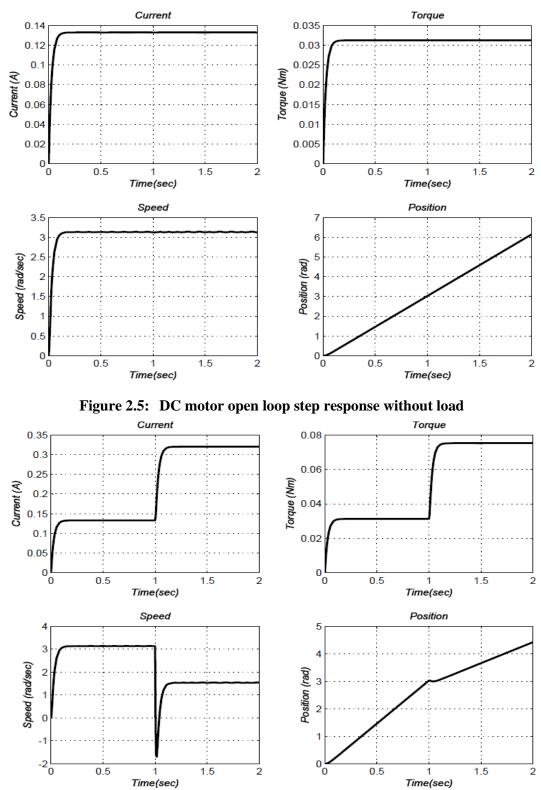
Simulation results using SIMULINK are shown in Figure 2.5 and Figure 2.6 for DC motor model with and without load disturbance.
