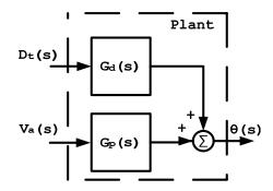
Figure 3.8: Servomotor model
