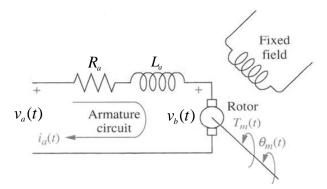
Figure 2.2: Schematic of DC motor system
