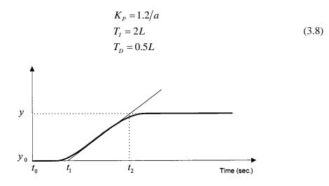
Figure 3.3: Plant step response in Z-N method
