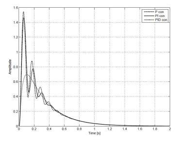
Figure 3.7: Transient response to step disturbance input
