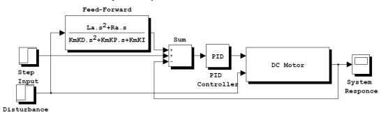
Figure 3.11: PID controller with feedforward compensator
