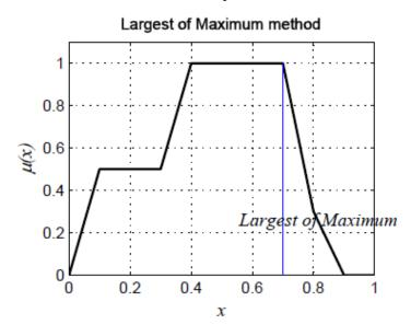
Figure C.4: Largest of Maximum defuzzification method
