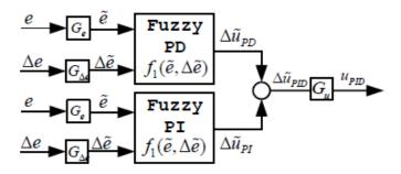
Figure 4.14: Two input fuzzy PID (Type I)
