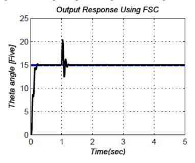
Figure 6.17: Output response using fuzzy supervisory control
