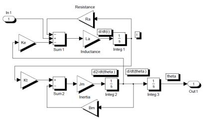
Figure 2.4: DC motor subsystem using SIMULINK
