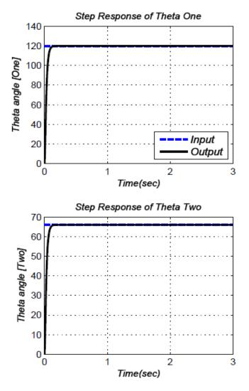
**Figure 6.5: PID** control step response for  $\theta_1, \theta_2$
