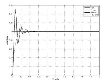
Figure 3.6: Transient response to step reference input
