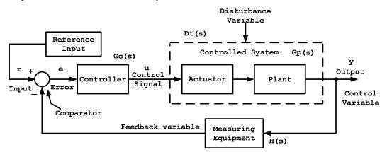
Figure 1.2: Block diagram of a closed-loop control system
