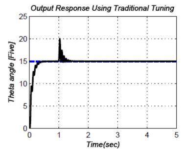
Figure 6.16: Output response using classical tuning methods
