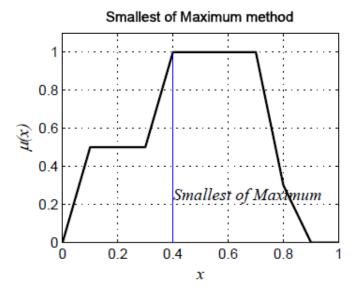
Figure C.5: Smallest of Maximum defuzzification method
