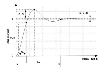
**Figure 3.5:** Unit step response curve showing  $t_r$ ,  $t_c$ , O.S and SSE
