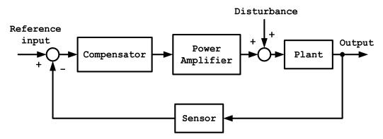
Figure 1.3: The basic structure of (SISO) system
