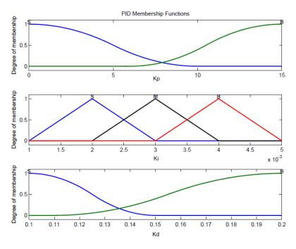
Figure 5.4: PID parameters membership functions
