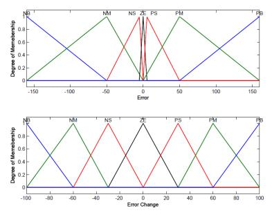
**Figure 4.8:** Membership function for inputs e and  $\Delta e$
