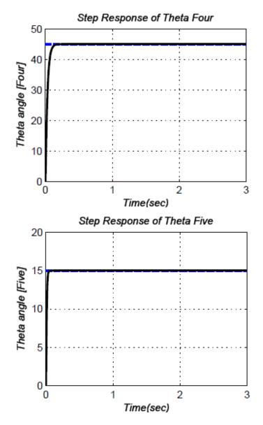
**Figure 6.7: PID control step response for**  $\theta_4$  and  $\theta_5$
