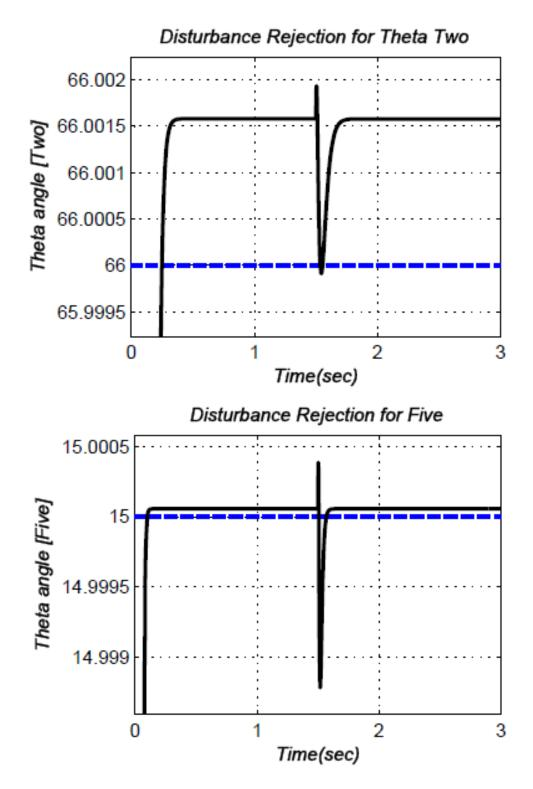
Figure 6.11: Output with disturbance rejection for  $\theta_2$  and  $\theta_5$
