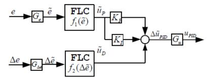
Figure 4.15: Two input fuzzy PID (Type II)
