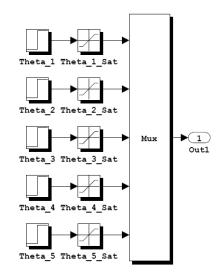
**Figure 3.13: Input angles with saturation boundaries**
