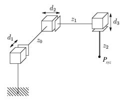
Figure 2.1: Robot manipulator with PPP joints [1]
