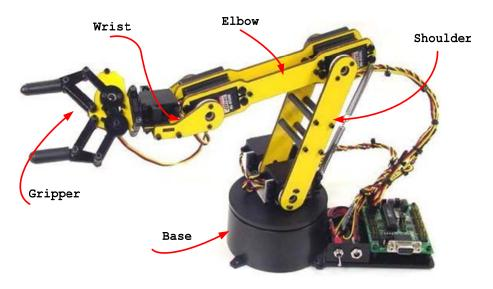
Figure 6.1: Lynx6 robot arm
