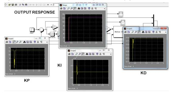
Figure D.5: Output response using FSC with PID parameter variations
