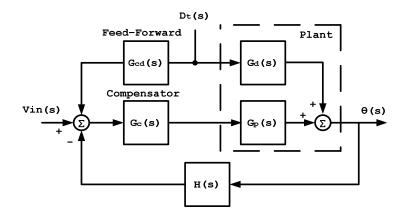
Figure 3.10: Feedforward compensation
