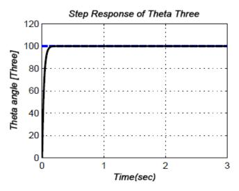
**Figure 6.6: PID control step response for**  $\theta_3$
