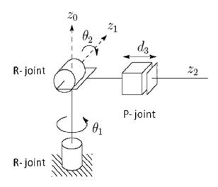
Figure 1.1: Manipulator with Revolute and Prismatic Joints [1]
