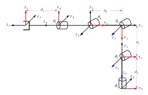
Figure 6.2: Frame assignment for the Lynx 6 robot arm.
