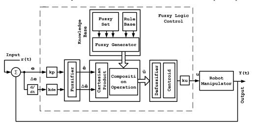
Figure 4.6: Fuzzy control system structure
