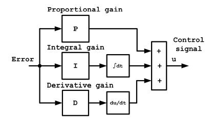
Figure 3.1: PID controller structure
