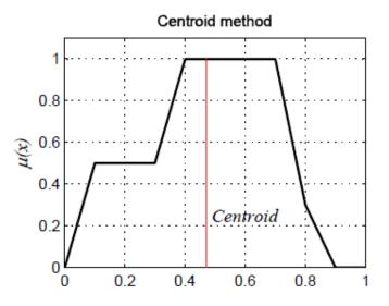
Figure C.1: Centroid defuzzification method
