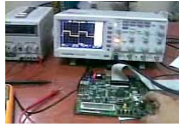
Fig. 25. Examining PWM output.
