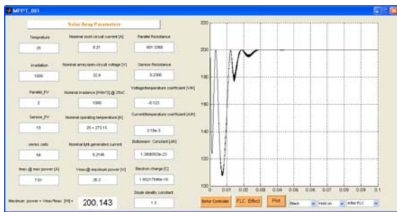
Fig. 19. GUI for entering parameters of any array from its datasheet.
