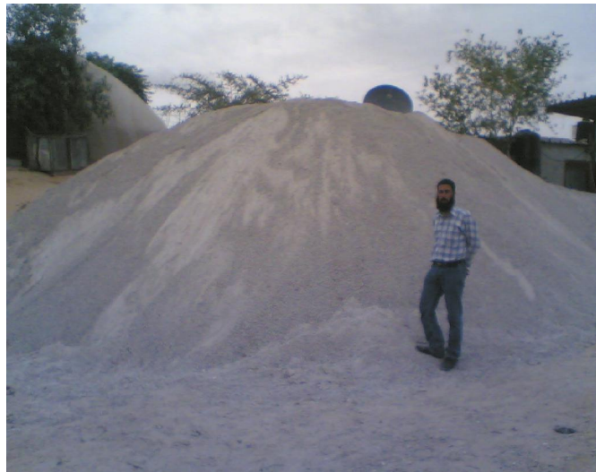
Figure 2.4: Stock piling of crushed demolished concrete fine aggregate in Gaza City
