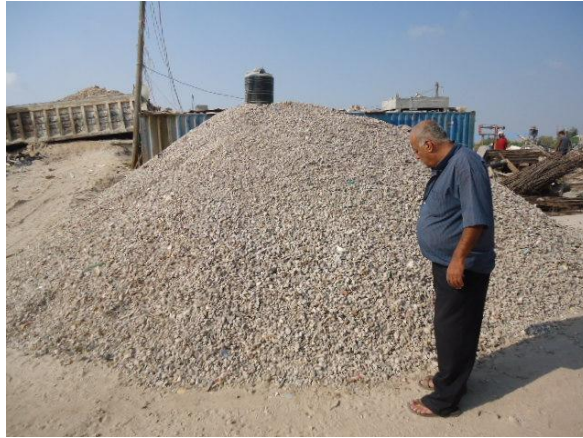
Figure 2.3: Stock piling of crushed demolished concrete coarse aggregate in Gaza City
