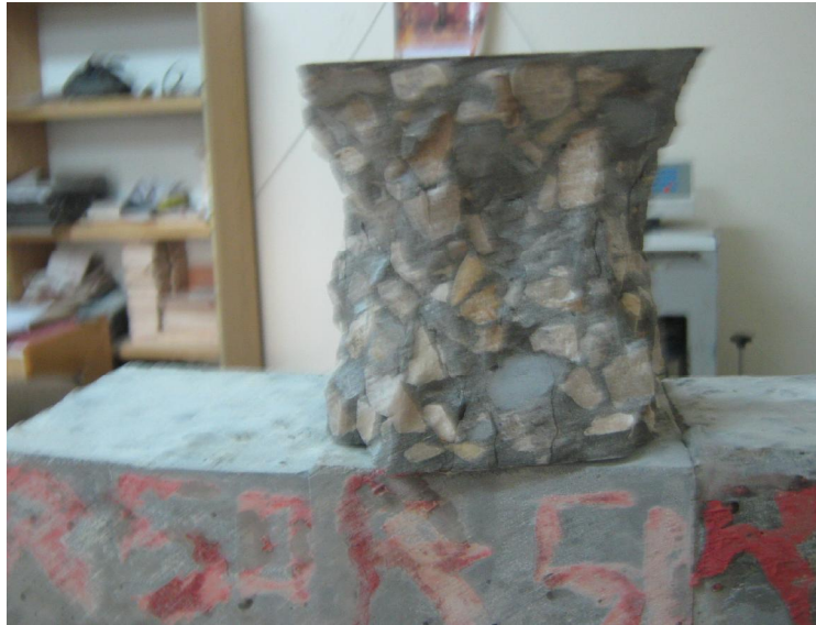
Figure 5.8: Typical testing cubs after failure for determine concrete compressive strength
