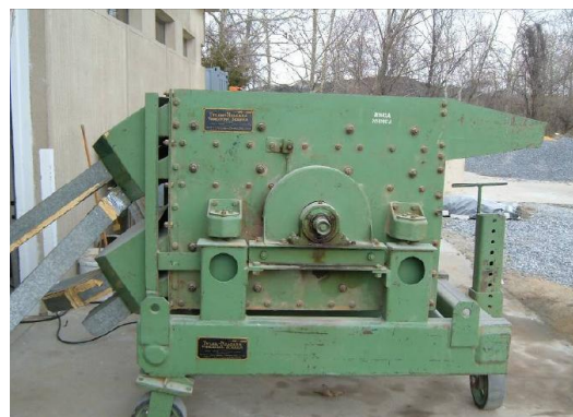
Figure 2.2: Large Capacity Sieve Shaker
