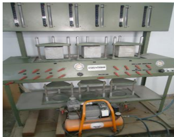
Figure 4.23: Water penetration test set-up
