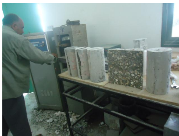
Figure 5.14: Illustration of splitting strength testing specimens after failure
