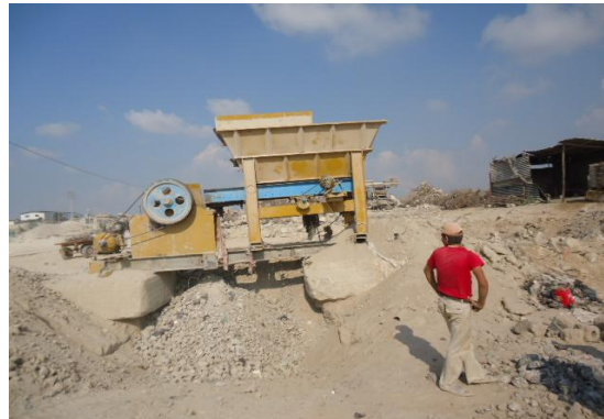
Figure 2.1b: Local crusher machine used to produce RAC at Gaza Strip
