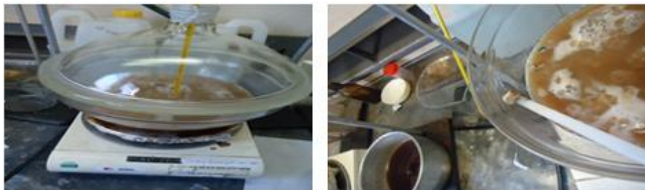
Figure 4.9a: RCA specimen placed in nitric solution and reaction
