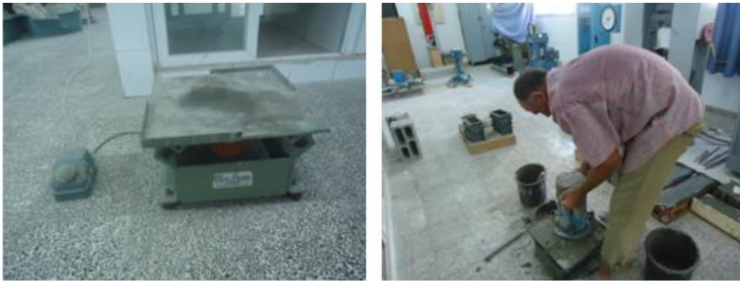
Figure 4.17: Illustration electrical vibration machine & casting samples
