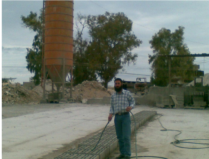
Figure 2.6: Shows new Hollow block product by utilization of RCA, in Gaza city
