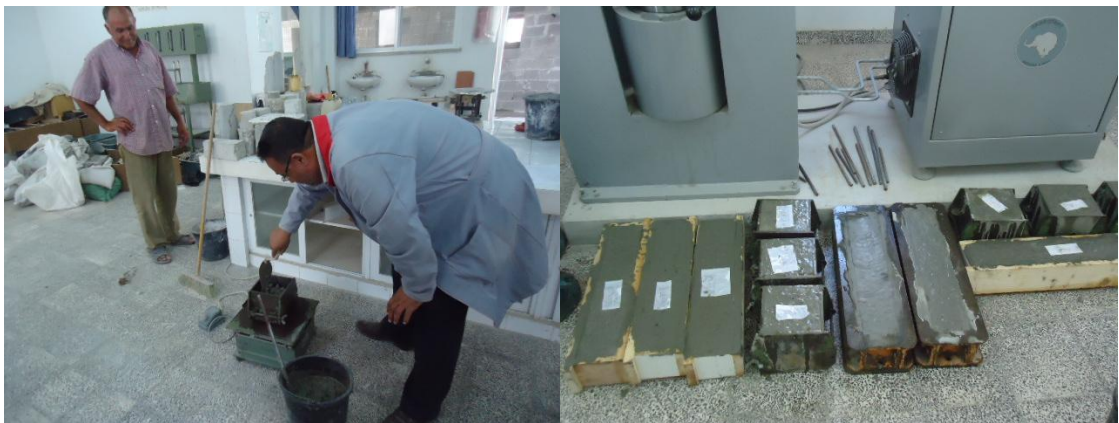
Figure C4:Oiling mold, casting and vibrating samples
