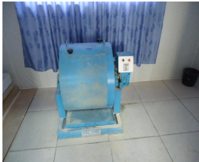
Figure 4.10 Loss Anglos instrument used for aggregate abrasion resistance test
