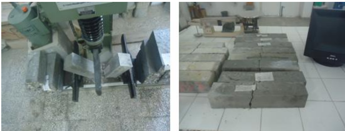
Figure 5.13: Illustration of days flexure strength testing specimens after failure
