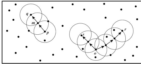
**Fig. 1.** Density reachability and density connectivity in density-based clustering (Source: Data Mining Concepts and Techniques, Secnd edition, p419)
