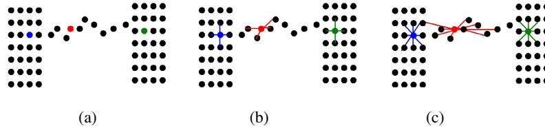
**Fig. 4.** (a) shows two clusters connected by a noise bridge, (b) using  $k=4$ , the noise point Eps value similar to the core points Eps, (c) increasing the value of  $k$ , will increase the Eps value of the noise
