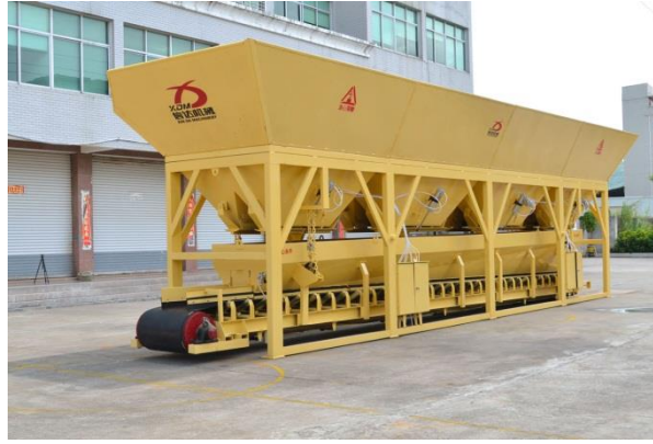
Figure (5.5): Aggregate bins and Belt Scale.
