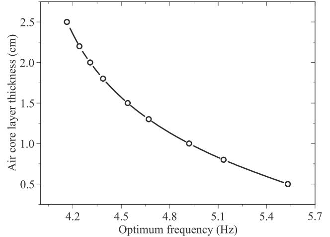
Fig. 4. Thickness of air core layer vs. the corresponding optimum frequency for TE<sub>1</sub> mode for  $\epsilon_{1x} = \epsilon_{1y} = 2.25$ , and  $\mu_{1x} = \mu_{1y} = 1$ ,  $F = 0.56$ ,  $\omega_o = 2\pi \times 4\text{GHz}$ ,  $\omega_p = 2\pi \times 10\text{GHz}$ ,  $\gamma = 0.012\omega_p$ ,  $\epsilon_2 = 1$ , and  $\mu_2 = 1$ .
