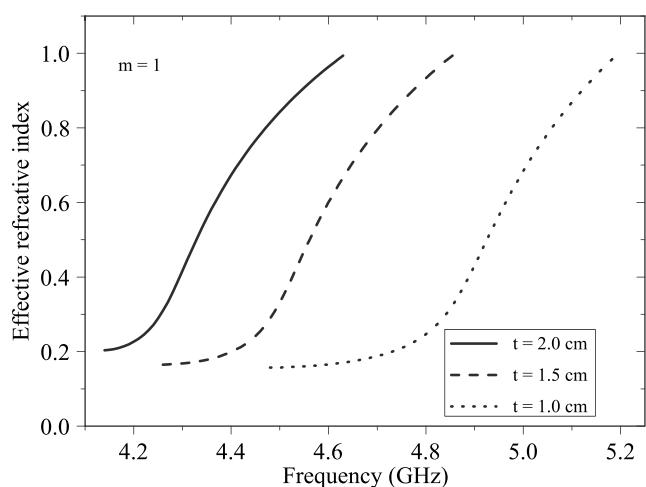
Fig. 2. Dispersion curves of the first guided mode ( $\text{TE}_1$ ) for different air film thicknesses for  $\epsilon_{1x} = \epsilon_{1y} = 2.25$ , and  $\mu_{1x} = \mu_{1y} = 1$ ,  $F = 0.56$ ,  $\omega_o = 2\pi \times 4\text{GHz}$ ,  $\omega_p = 2\pi \times 10\text{GHz}$ ,  $\gamma = 0.012\omega_p$ ,  $\epsilon_2 = 1$ , and  $\mu_2 = 1$ .
