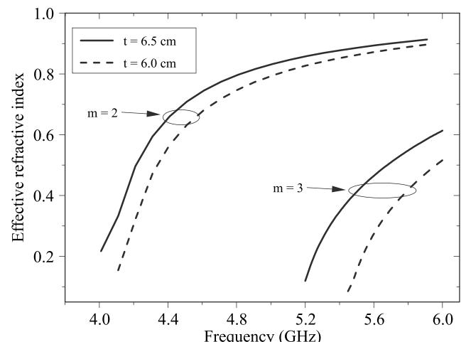
Fig. 5. Dispersion curves of the second and third guided modes (TE<sub>2</sub> and TE<sub>3</sub>) for different guiding film thicknesses for  $\epsilon_{1x} = \epsilon_{1y} = 2.25$ , and  $\mu_{1x} = \mu_{1y} = 1$ ,  $F = 0.56$ ,  $\omega_o = 2\pi \times 4\text{GHz}$ ,  $\omega_p = 2\pi \times 10\text{GHz}$ ,  $\gamma = 0.012\omega_p$ ,  $\epsilon_2 = 1$ , and  $\mu_2 = 1$ .
