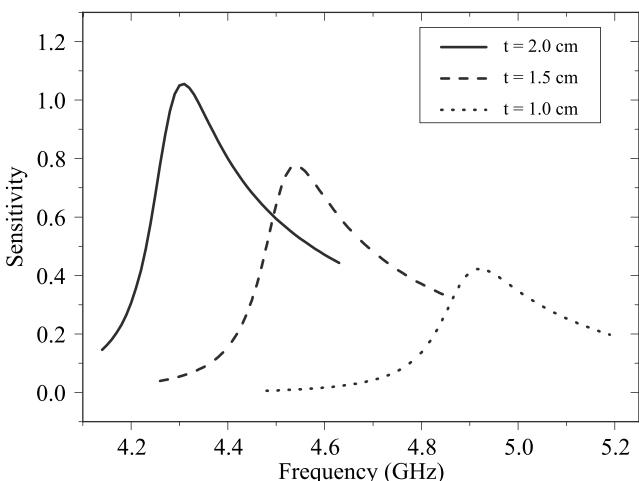
Fig. 3. Sensitivity as a function of the angular frequency for TE<sub>1</sub> mode for different guiding film thicknesses for  $\epsilon_{1x} = \epsilon_{1y} = 2.25$ , and  $\mu_{1x} = \mu_{1y} = 1$ ,  $F = 0.56$ ,  $\omega_o = 2\pi \times 4\text{GHz}$ ,  $\omega_p = 2\pi \times 10\text{GHz}$ ,  $\gamma = 0.012\omega_p$ ,  $\epsilon_2 = 1$ , and  $\mu_2 = 1$ .
