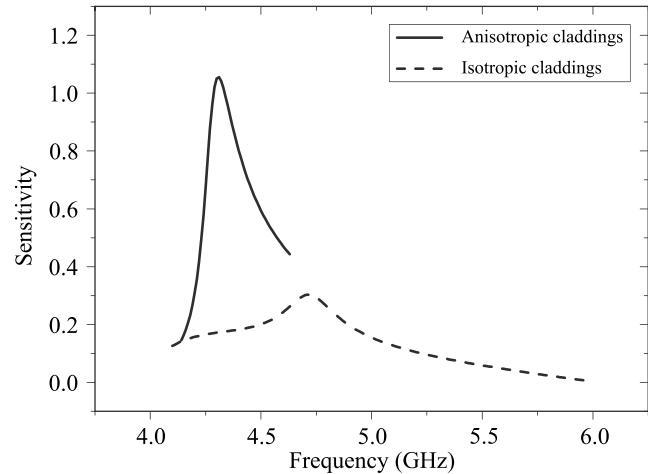
Fig. 7. Sensitivity as a function of the angular frequency for TE<sub>1</sub> mode when the claddings are anisotropic (solid line) and when the LHM anisotropy is neglected (dashed line).
