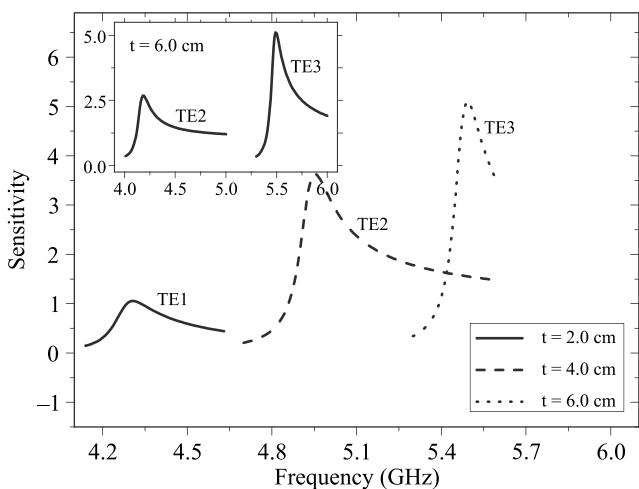
Fig. 6. Sensitivity as a function of the angular frequency for different guided modes for  $\epsilon_{1x} = \epsilon_{1y} = 2.25$ , and  $\mu_{1x} = \mu_{1y} = 1$ ,  $F = 0.56$ ,  $\omega_o = 2\pi \times 4\text{GHz}$ ,  $\omega_p = 2\pi \times 10\text{GHz}$ ,  $\gamma = 0.012\omega_p$ ,  $\epsilon_2 = 1$ , and  $\mu_2 = 1$ .
