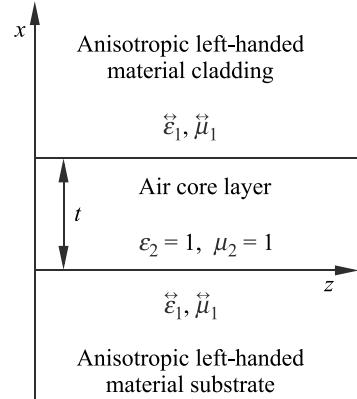
Fig. 1. A three-layer slab waveguide structure including air core layer and anisotropic left-handed material claddings.
