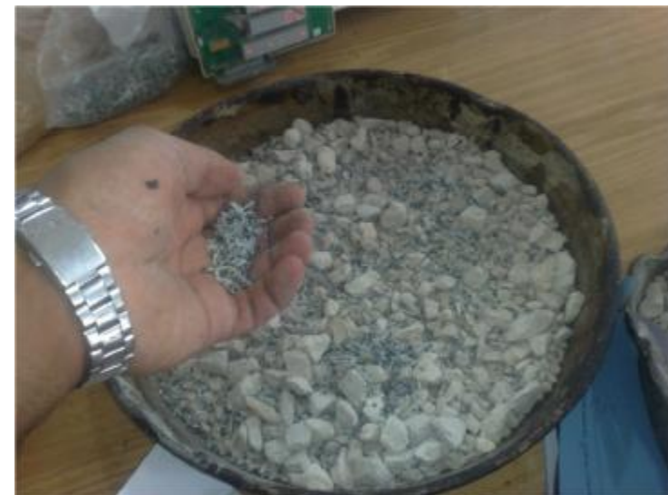
Figure (F.8): Adding WPB to the Aggregates
