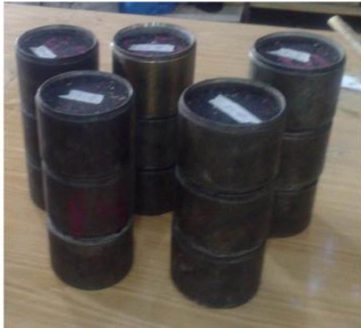
Figure (F.5): Job mix Marshal Samples
