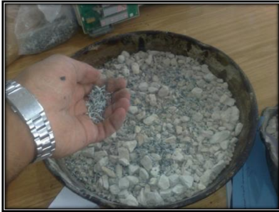
Figure (3.15): Adding WPB to aggregates before heating
