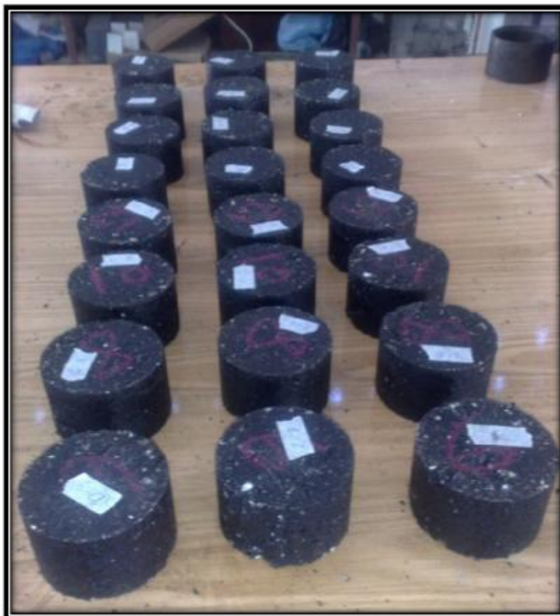
Figure (3.16): WPB modified Marshal Specimens
