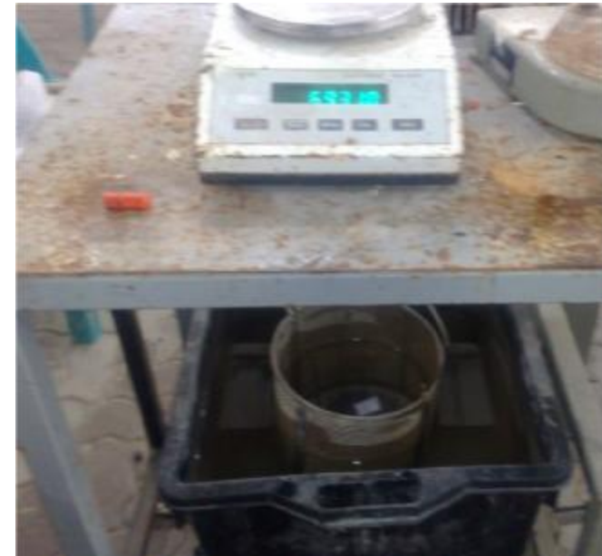
Figure (F.6): Marshal Samples weighing in water
