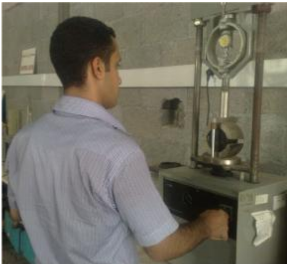
Figure (F.11): Testing Marshal Samples for stability and flow
