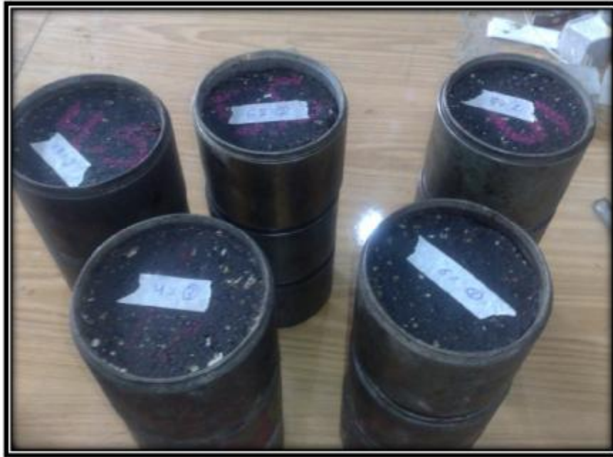
Figure (3.14): Marshall specimens for different bitumen percentages
