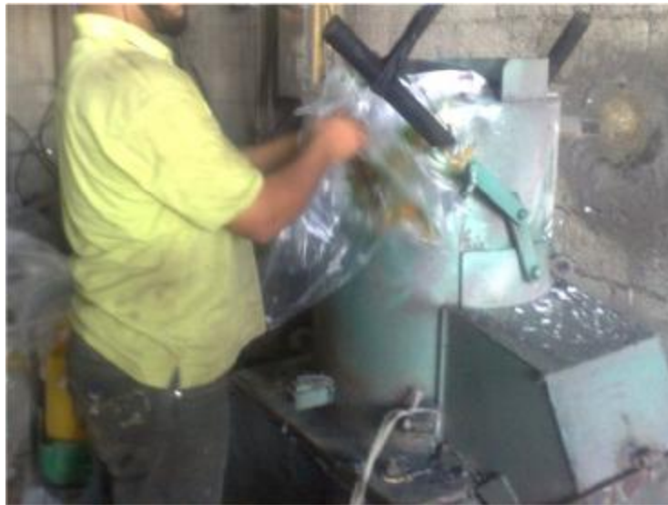
Figure (F.3): Waste plastic grinding
