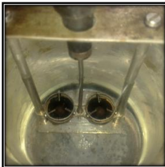
Figure (3.5): Softening point test for bitumen samples
