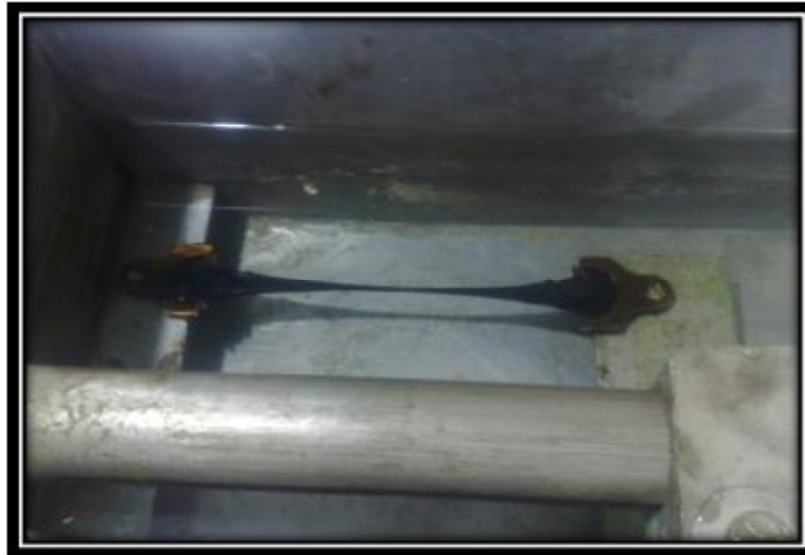
Figure (3.4): Ductility test for a bitumen sample
