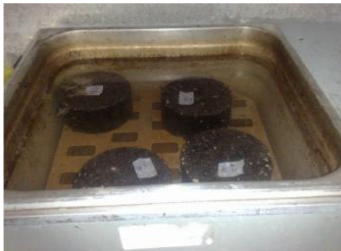
Figure (F.2): Water bath for Marshal Samples
