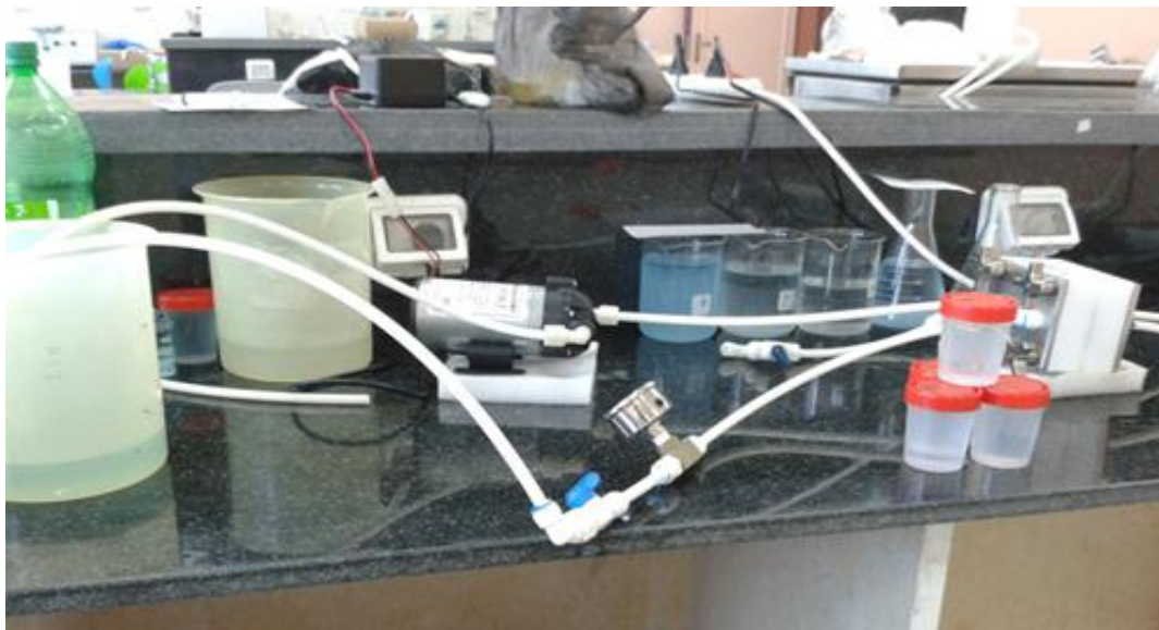
Figure (3.5): The lab scale experimental system for FO process
