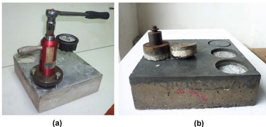
Figure 11. Failure of pull-off test through NC substrate. (a) Pull-off test setup and (b) failure of pull-off test.
