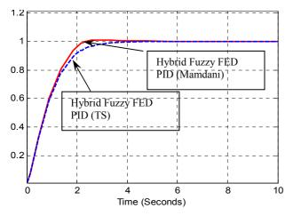
Fig.5: Stabilization control of the FED PID (M) versus FED PID (T-S)
