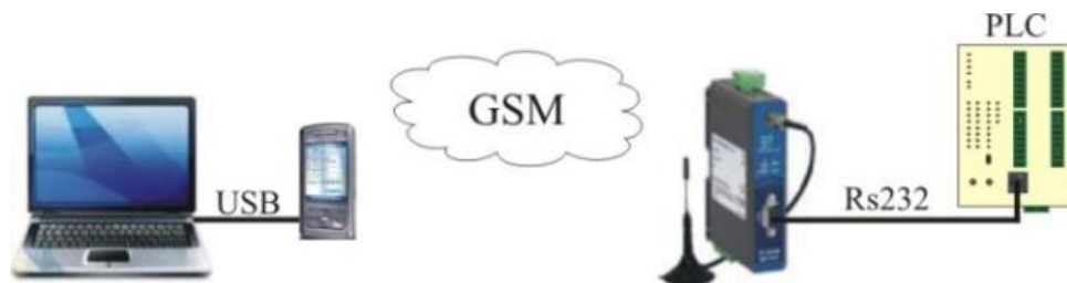
Figure (6.8): PLC cellular system connection
