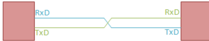
Figure (4.1): The two-wire RS-232 configuration
