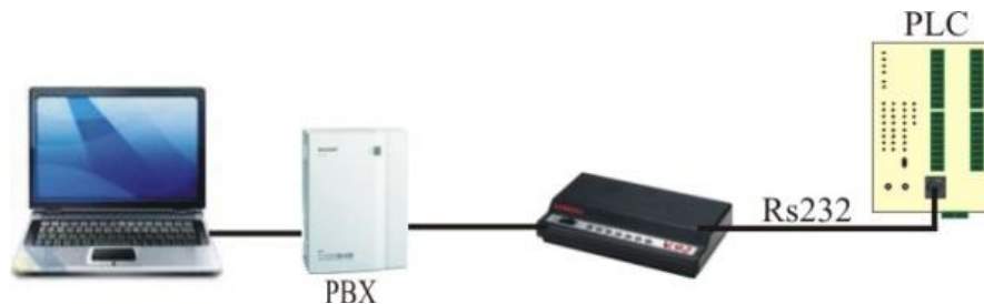
Figure (6.7): PLC dial up connection
