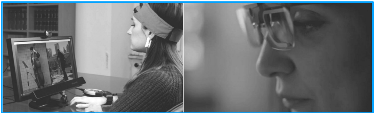
Figure 12. Example of eye trackers, fixed (left) and mobile (glasses, on the right). ( www.brainsigns.com )
