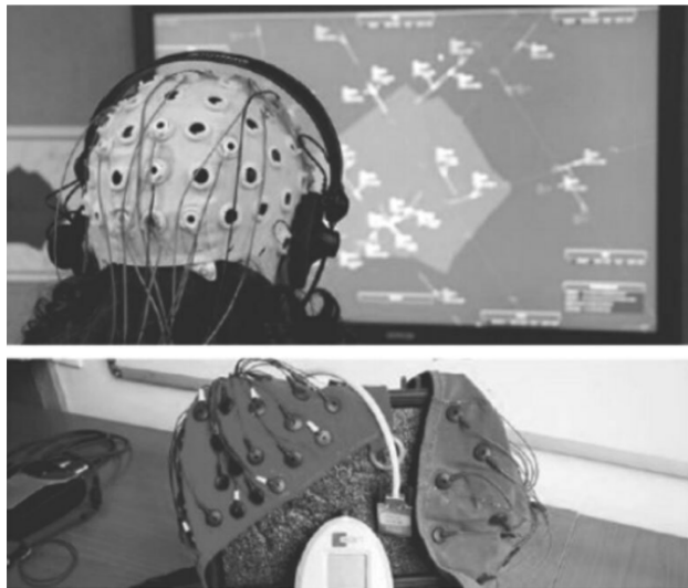
Figure 10. Standard EEG headset with 32 or 64 electrodes (BrainSigns, IN: Cherubino and Pozharliev, 2020)
