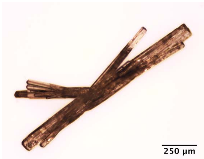
Figure 1 – Optical micrograph of Ce 2 (NDC) 3 (DMF) 2 crystals.
