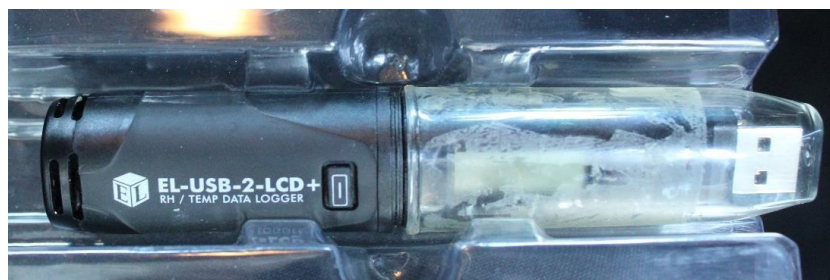
Figure 8: Datalogger "EL-USB-2-LCD+" Lascar Eletronics.
