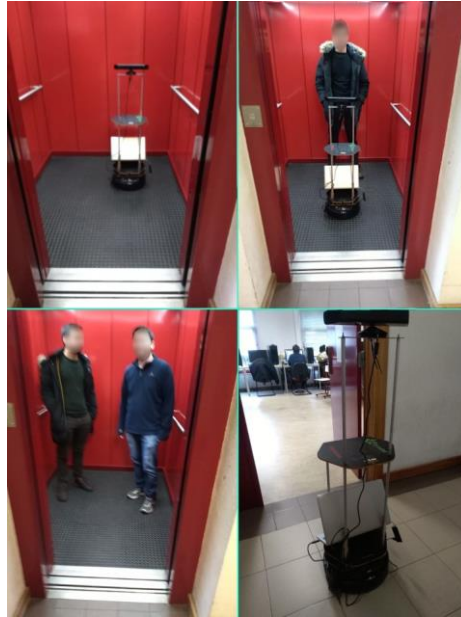
Figure 9.4: Robot entering an empty elevator; Robot entering an elevator with one passenger; Robot entering an elevator with two passengers; Robot entering a room.
