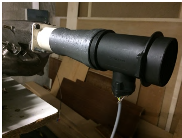
Figure 4.13: Inlet manifold-MAF sensor assembly.
