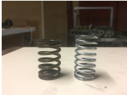
Figure 4.10: Original engine spring on the left along with the used spring.
