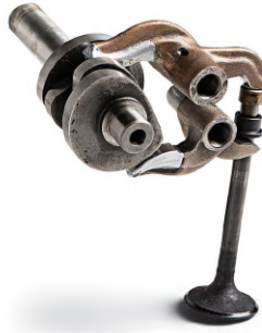
Figure 3.9: Desmodromic valve system [35].
