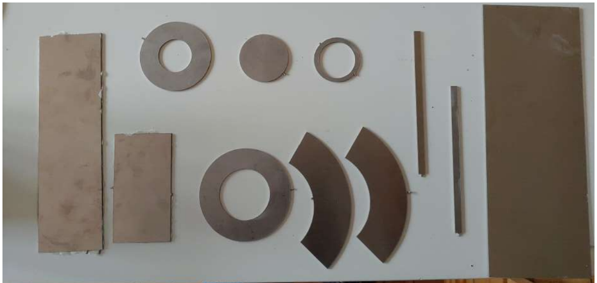
Figure 4.39: Samples of the pieces cut with the water jet
