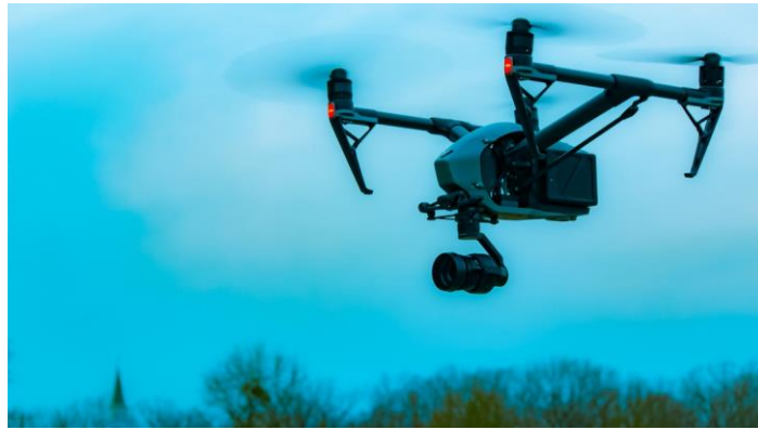
Figure 6 - Quadcopter UAV with an installed gimbal - Source: [21]
