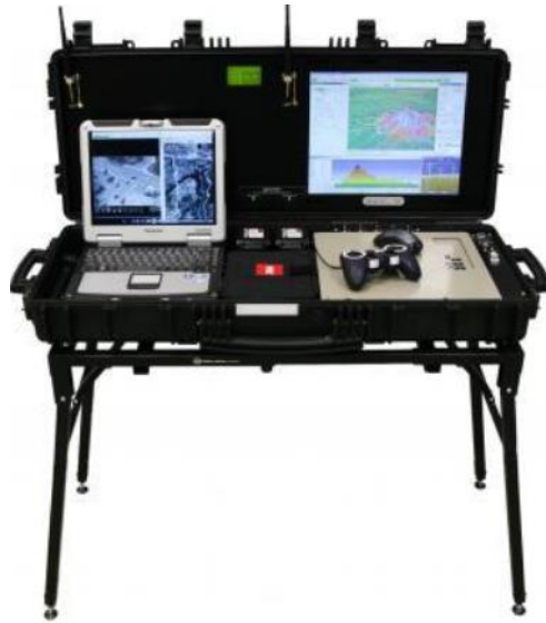
Figure 2.10 - Portable Ground Station by UAV Factory [23]
