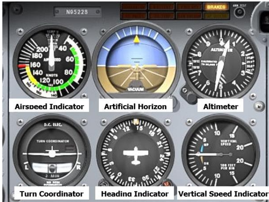
Figure 3.7 - Traditional Six Pack [Adapted from 46]
