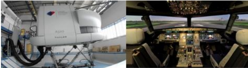
Figure 2.5 - A320 Full Flight Simulator (FFS), outside (left), and inside (right) [12]
