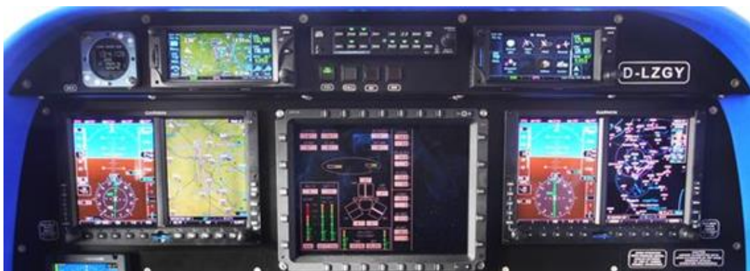
Figure 2.7 - Zeppelin's Flight Instruments [18]
