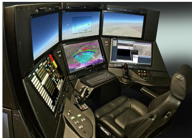
Figure 2.11 - Advanced Cockpit Ground Control Station (GCS) [24]
