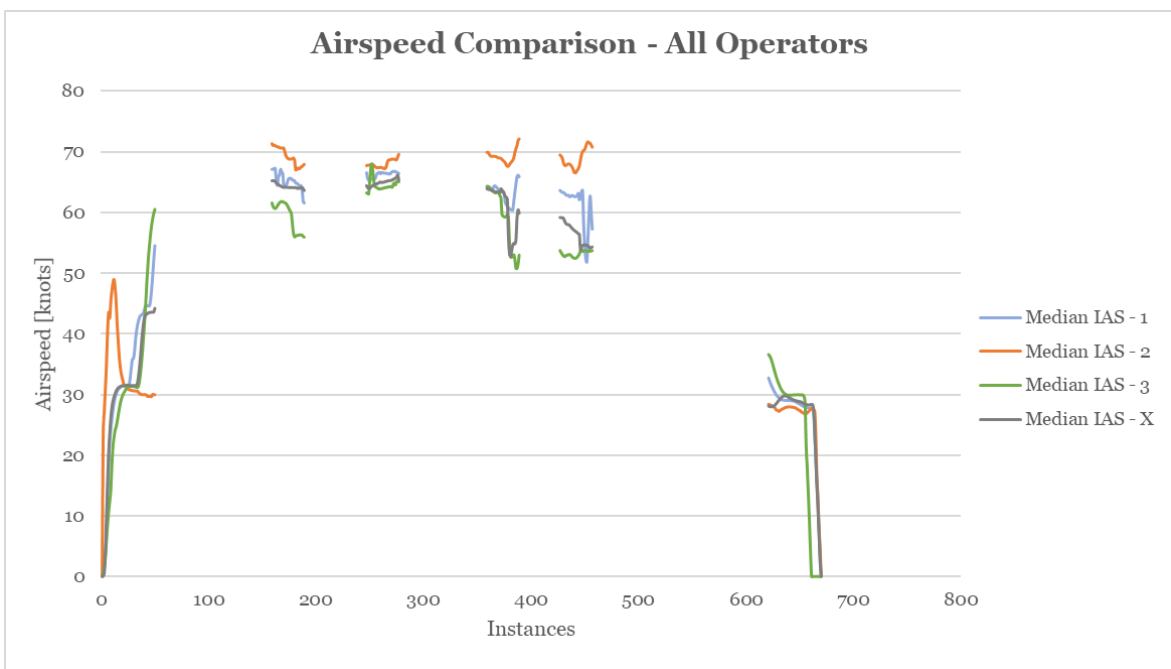
Figure 4.33 - Comparison of airspeed median values for all Operators per task
