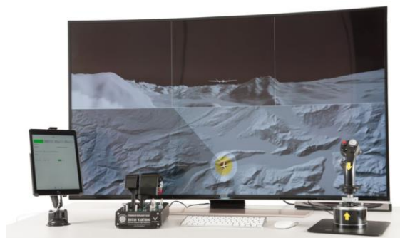
Figure 2.9 - Remote Pilot Station prototype with a panoramic screen [22]
