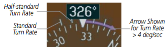
Figure 2-17 Turn Rate Indicator and Trend Vector
