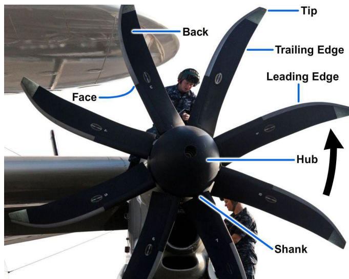
Figure 2.14 – Components of a propeller (NAVEDTRA, 1991)
