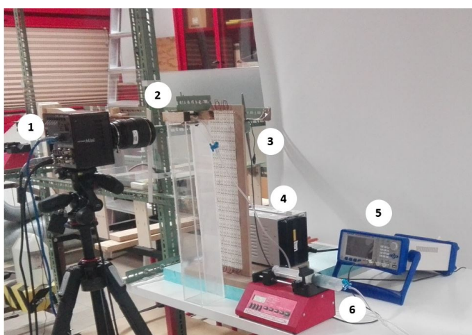
Figure 2.13: Experimental arrangement: 1) High speed camera; 2) Droplet generator; 3) Lighting source; 4) Power supply; 5) Signal generator; 6) Syringe pump.
