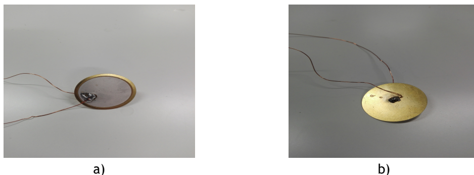
Figure 2.2: Piezoelectric diaphragm: a) front view; b) back view.
