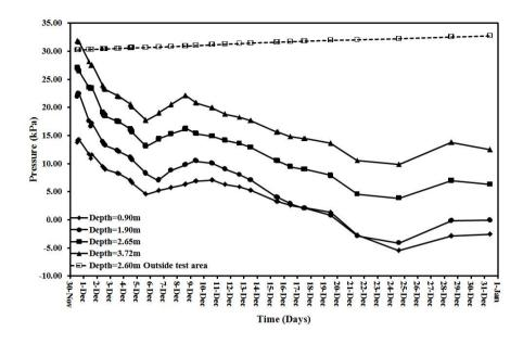
Figure 7 – Pore-water pressure variation for 1.20m PVD spacing subarea
