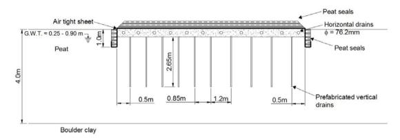
Figure 1 - Cross section of TCD/NRA vacuum preloading field trial
