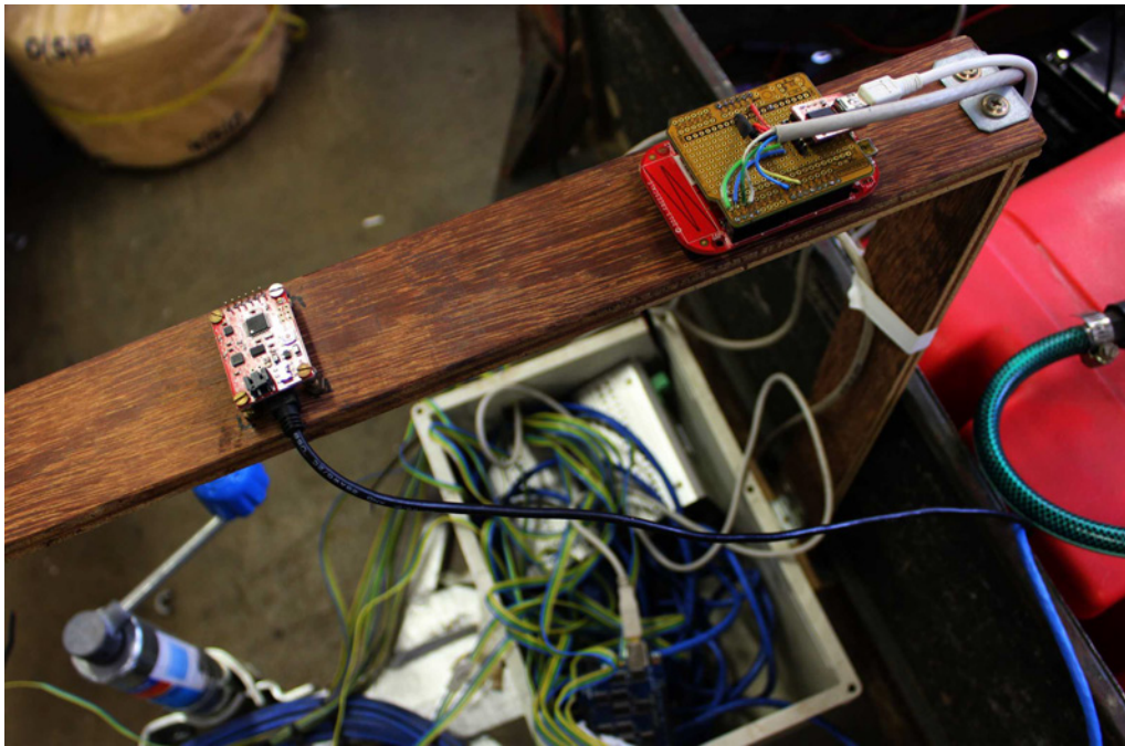
Figure 2.19: The IMU mounted in-place on the proof of concept vehicle.
