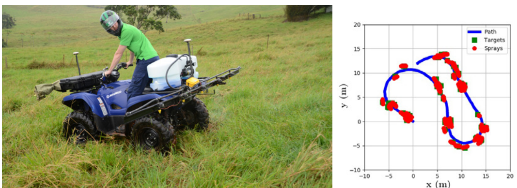
Figure 5.49: Left: Alex Olsen operating the AutoWeed spot-spraying prototype on a cattle station 10 km southeast of Malanda. Right: Location data for the Malanda trial.
