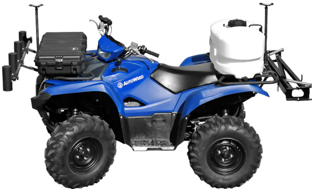
Figure 3.3: AutoWeed : A prototype weed control robot for selective foliar spot spraying in the Australian rangelands.
