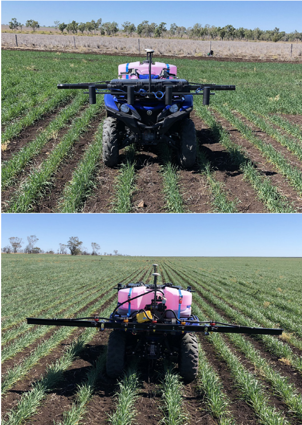
Figure 5.4: Front (top) and back (bottom) views of the AutoWeed spot-spraying prototype photographed during a field trial on a sowthistle infested wheat crop in Arcturus Downs, QLD.
