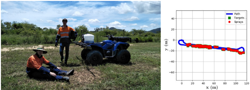
Figure 5.48: Left: Alex Olsen and Brendan Calvert operating the AutoWeed prototype in Townsville. Right: Location data for the Townsville trial.
