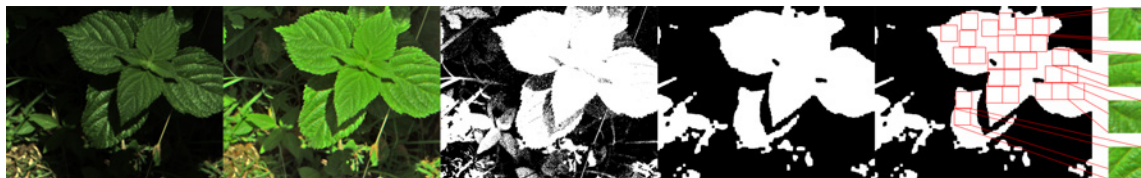
Figure 2.7: An example of our leaf area segmentation algorithm. Left to right: Input image, contrast normalised output, RGB thresholding output, morphological opening and closing output, final result superimposed with extracted windows.
