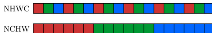
Figure 4.31: A simplified representation of the two most common tensor formats, NHWC, the TensorFlow default format and NCHW, the TensorRT default format.
