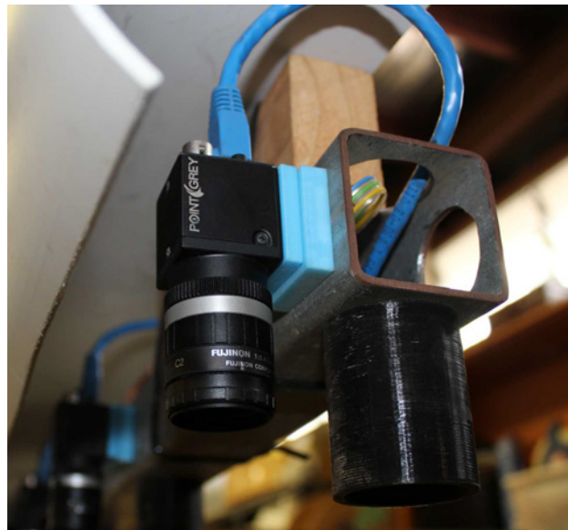
Figure 2.21: Photograph of the chosen camera and lens optical system mounted to the proof of concept.
