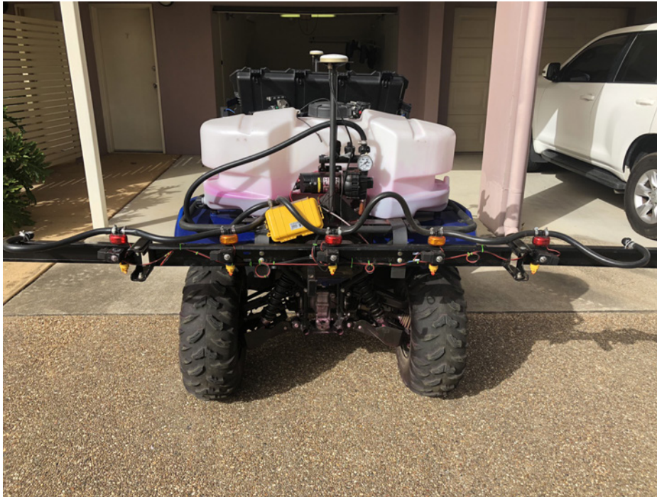
Figure 5.26: Developed AutoWeed prototype sprayer system with 35 cm spaced solenoids and LED indicators above each nozzle.
