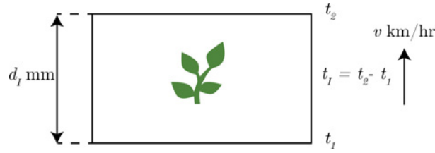
Figure 4.28: An illustration of the first real time speed limitation whereby the time it takes to process an image must not exceed the time it takes to traverse its field of view.
