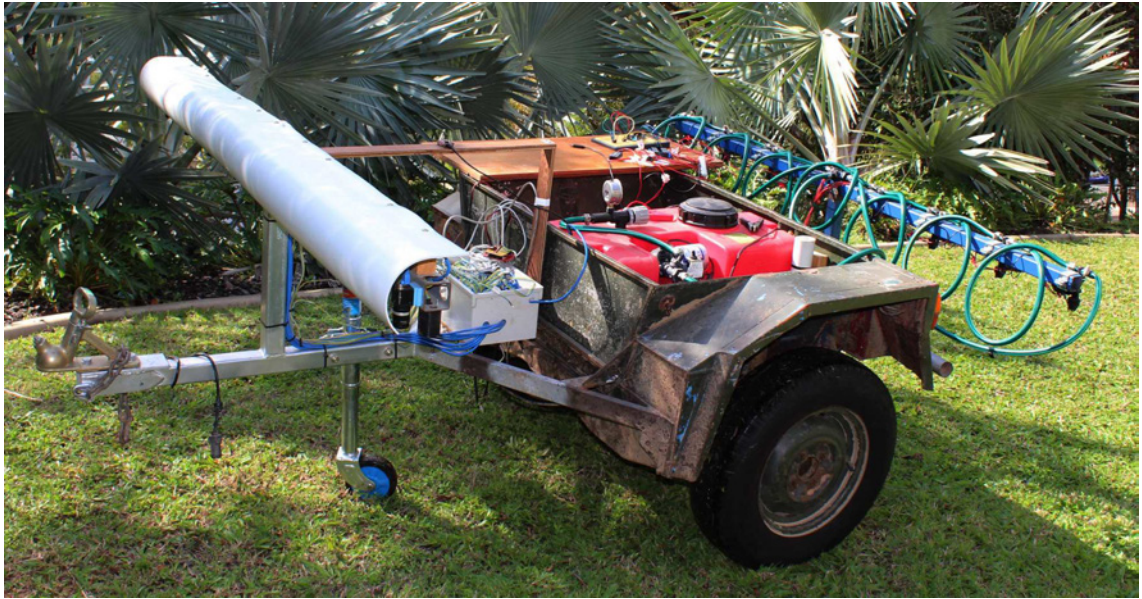
Figure 2.18: Completed design of the proof of concept weed detection and spot spraying system mounted to a towable trailer.
