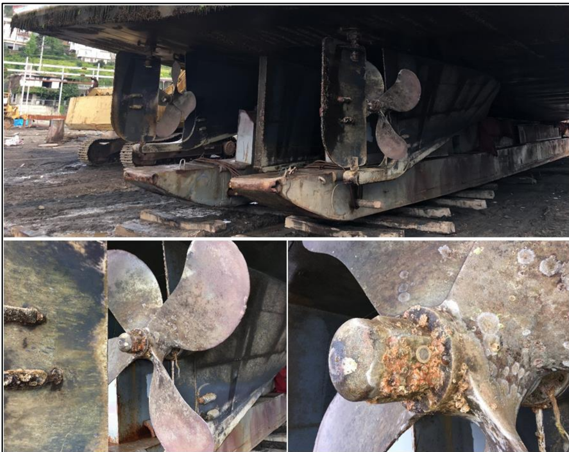
Figure 1 Biofouling after a year of operation on a propeller
