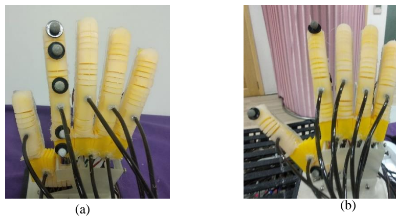
Figure 4. The soft robot hand: (a) palm side, (b) back side, and (c) soft robot hand with fingertip haptic feedback for teleoperation.
